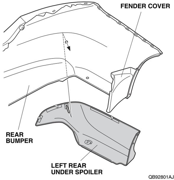
22. Loosely install one bolt, one spring nut, and one new self-tapping screw.
