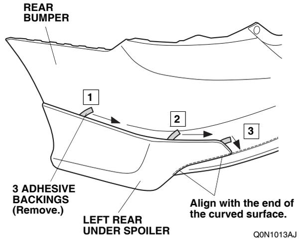
25. Remove three adhesive backings in the order shown. Press the left rear under spoiler firmly against the rear bumper with the palm of your hand for 30 seconds to adhere the left rear under spoiler.
