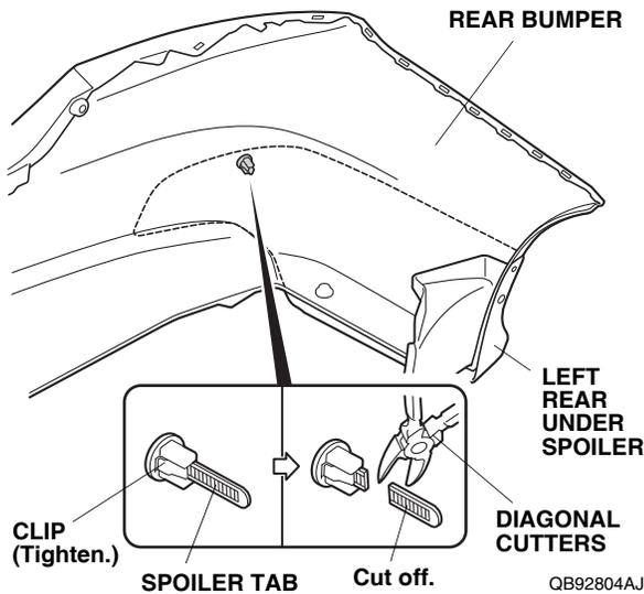
27. Using diagonal cutters, cut the excess off of the spoiler tab.
