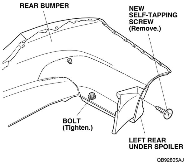
29. Remove one new self-tapping screw loosely installed in step 22.
