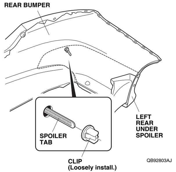
24. Align the left rear under spoiler with the rear bumper as shown.
