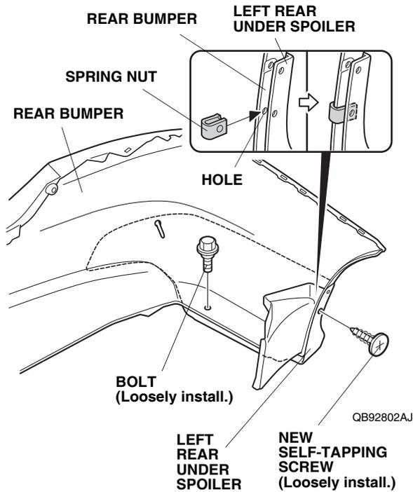
23. Loosely install a clip to the spoiler tab.
