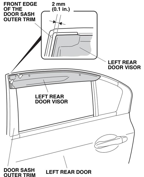
19. While applying light pressure against the left rear door visor, carefully remove the adhesive backings. Use your finger to push up each bracket so there is no gap between the brackets and the door sash.
