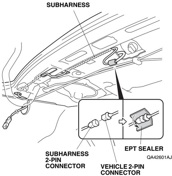
35. Align the green tape on the subharness with the vehicle clip, and secure the subharness to the vehicle harness with one wire tie.
