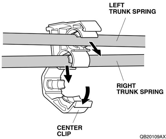
24. Put on heavy gloves to protect your hands. With an assistant holding the trunk lid open, remove both trunk springs with the trunk spring tool. Pull the trunk spring tool slowly and carefully toward you. First remove the right trunk spring, then remove the left trunk spring.
