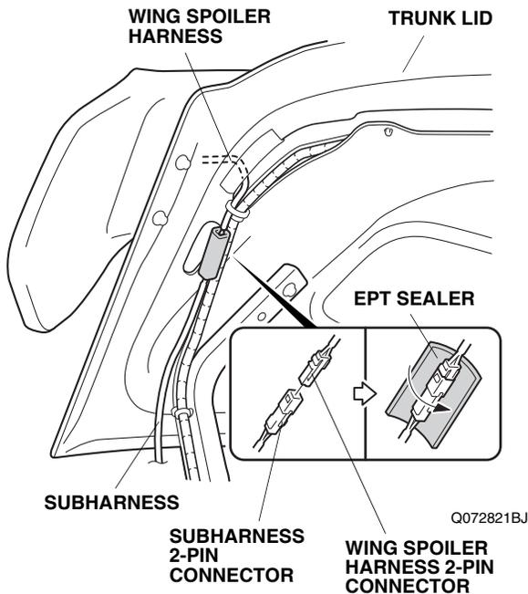
38. Secure the subharness to the vehicle harness with three wire ties in the area shown. Do not secure the wire tie to the trunk opener cable.
