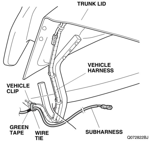
36. Connect two wire ties together and secure the subharness to the vehicle panel with the connected wire tie.
