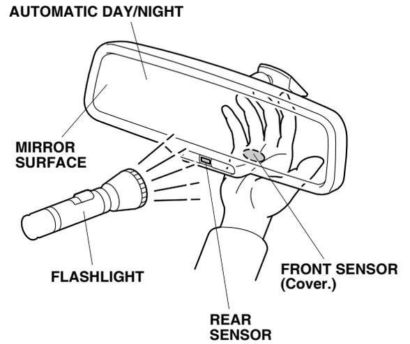
4. Step on the brake pedal, and move the select lever to the "R" position. Repeat step 3, and check to make sure the mirror surface does not become dim.
