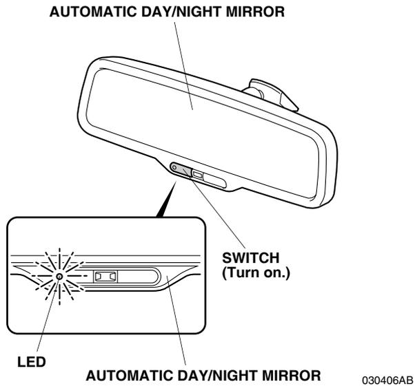
2. Turn the switch on. Check that the LED lights.
