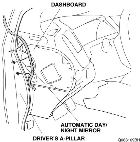
34. Align the green tape on the automatic day/night mirror harness with the vehicle clip, and secure the automatic day/night mirror harness to the vehicle harness with one wire tie A.
