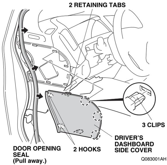
15. Remove the driver's dashboard side cover (three clips, two retaining tabs, and two hooks).
