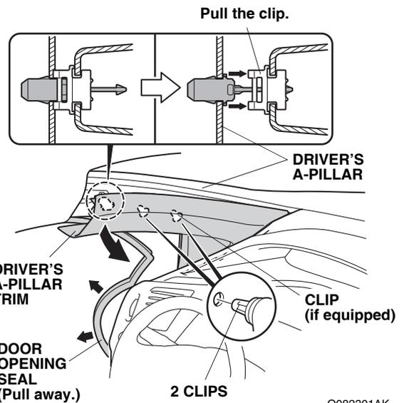
9. Pull out the driver's A-pillar trim to release the clips.
