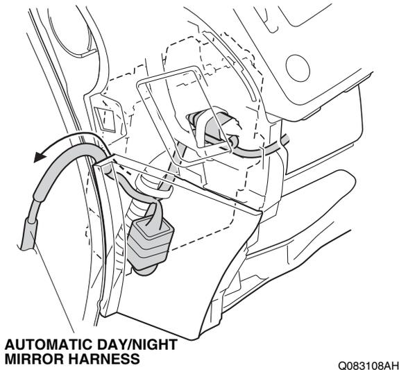
33. Insert the automatic day/night mirror harness between the dashboard and the driver's A-pillar.
