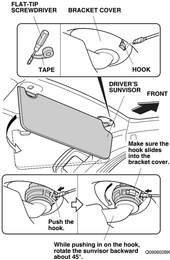
6. While pushing in on the hook, rotate the driver's sunvisor backward about 45°. Make sure the hook slides into the bracket cover.
