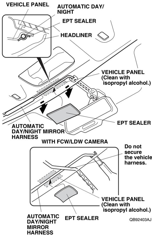
41. Secure the automatic day/night mirror harness to the vehicle panel with one EPT sealer as shown. Be careful not to crease the headliner.
