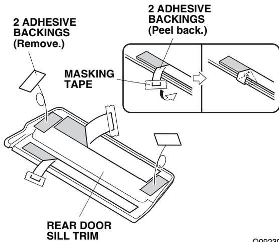
65. Position the rear door sill trim with the masking tape.
