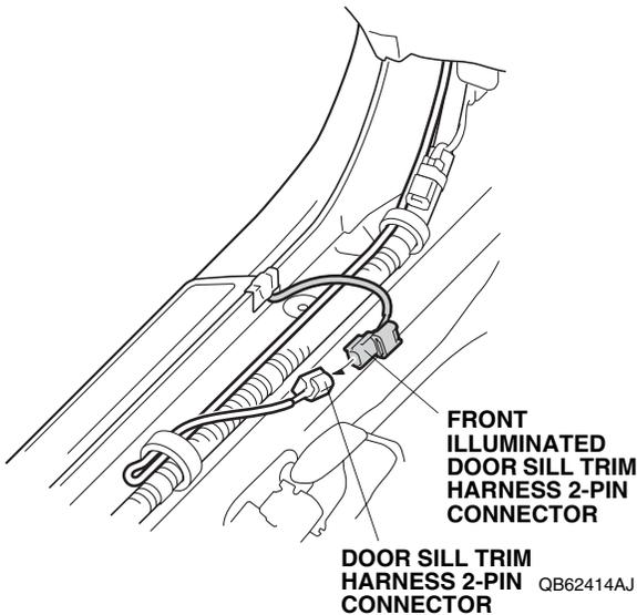
45. Bundle up the excess front illuminated door sill trim harness, and secure it to the vehicle harness with one wire tie with holder.
