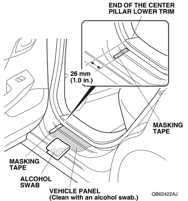
62. Attach a strip of masking tape to the vehicle panel at the measurement shown.
