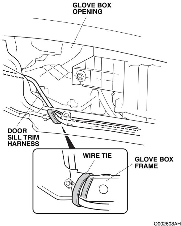
26. Inside the center lower panel opening, secure the door sill trim harness to the vehicle harness with two wire ties.
