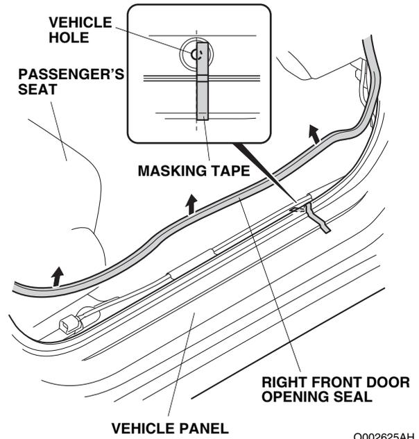
47. Attach a strip of masking tape to the vehicle panel at the location shown.
