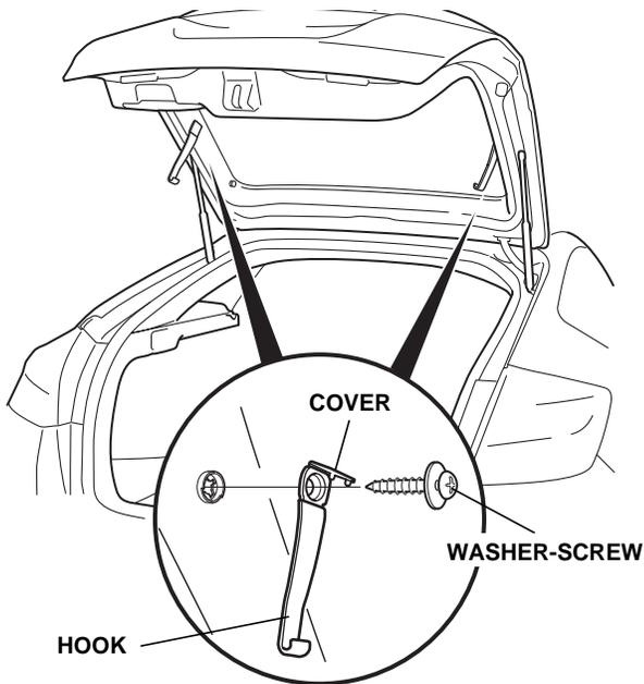
3. Snap the tailgate liner onto the hooks. Align the pins on the tailgate liner with the holes in the tailgate, then push on the liner to seat the pins.
