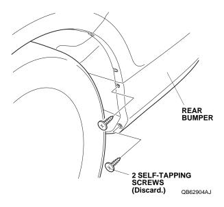
6. Install the left rear splash guard onto the rear bumper with two self-tapping screws, and tighten them in the order shown.
