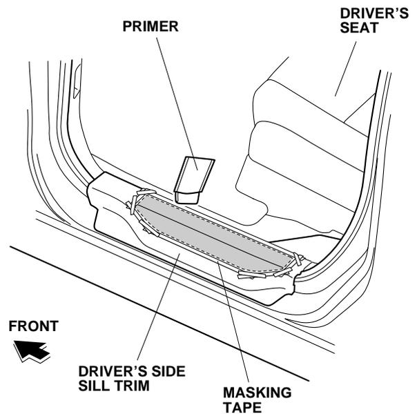
5. Allow the primer to dry for at least three minutes. **NOTE:** Make sure you allow the primer to dry thoroughly before continuing with the next step. Re-apply the primer if 24 hours have passed since the primer was applied.
