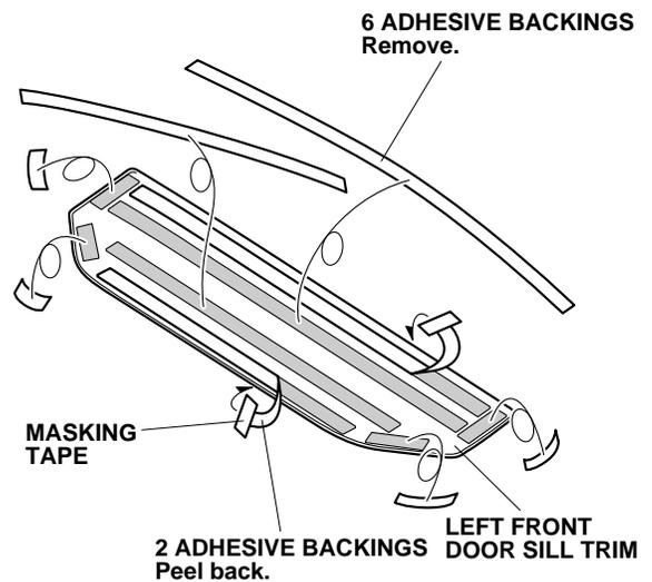
8. Remove the remaining adhesive backings.
