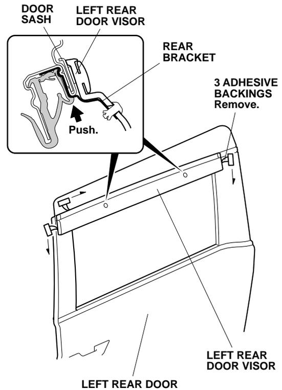
20. Using the palm of your hand, firmly press the left rear door visor against the door sash.
