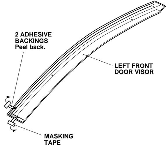
6. Place the door visor against the door, and adjust the visor so it lines up with the two front brackets.
