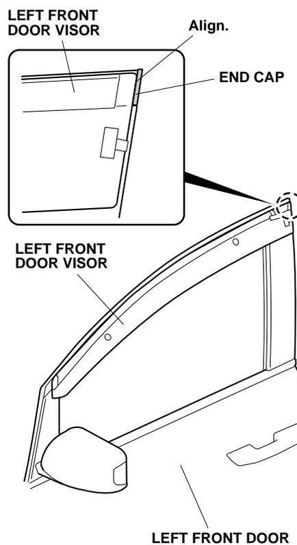
9. While applying light pressure against the left front door visor, carefully remove the adhesive backings. Push up on the front brackets while removing the adhesive backings.
