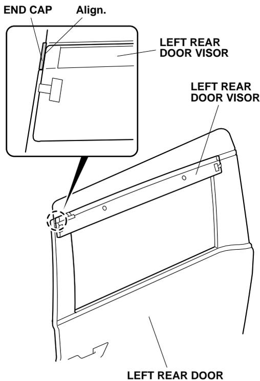
19. While applying light pressure against the left rear door visor, carefully remove the adhesive backings. Push up on the rear brackets while removing the adhesive backings.
