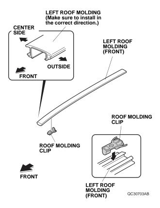
Reinstall the roof molding left cover.
