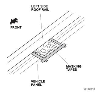
17. Hook the left center roof rail cover to the left side roof rail as shown.
