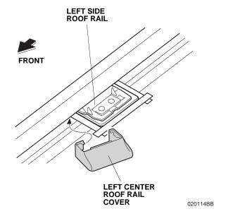
18. Install the left center roof rail cover to the left side roof rail as shown. Make sure that the left center roof rail cover is no clearance between the left side roof rail.
