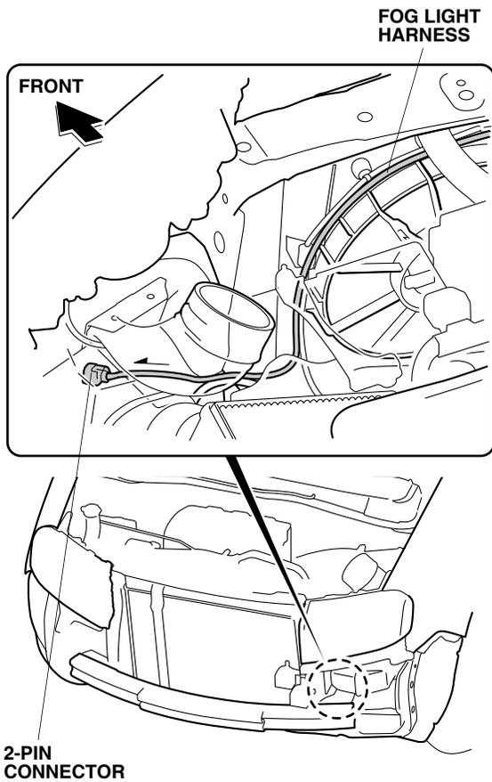
22. Secure the clip on the fog light harness to the vehicle panel hole.
