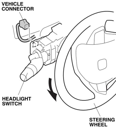
31. Remove two self-tapping screws from the headlight switch. While pushing the retaining tab, remove the headlight switch from the steering column. NOTE: Do not pull on the lever when removing the switch.
