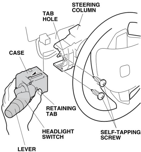
32. Hold the retaining tab, then install the new headlight switch to the steering column. Secure it with the two self-tapping screws. NOTE: Do not push on the lever when installing the case.
