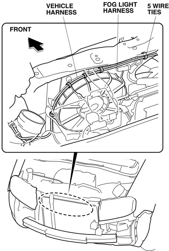
26. With the help of an assistant, bring the front bumper to the vehicle, and plug two fog light harness 2-pin connectors to two fog lights. Reinstall the front bumper.
