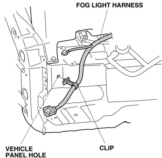
18. Route the other end of the fog light harness 2-pin connector along the vehicle harness.
