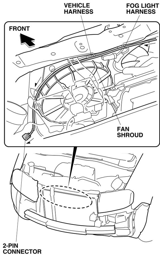
21. Continue to route the fog light harness 2-pin connector down and through the front bulkhead.
