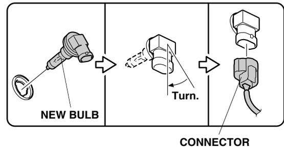
5. Reinstall the removed parts. Check that the wire harnesses are not pinched. Be sure to tighten the clip and bolts securely.
