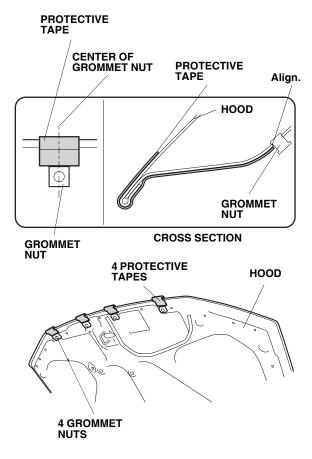
3. Remove the adhesive backings from each protective tape and attach the four protective tapes around the front of the hood as shown.
