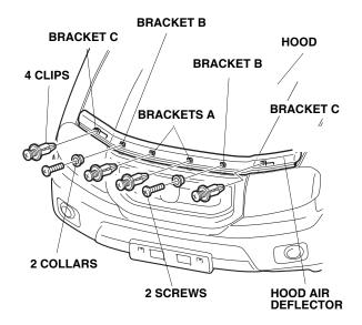
14. Insert the large end of the template between the hood and the hood air deflector to unfold the molding as necessary.
