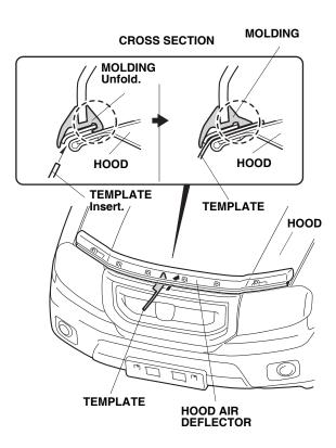
15. Open the hood. Tighten the four truss screws loosely installed in step 4.
