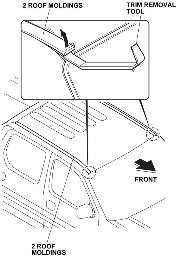
2. Slide and remove the two roof moldings from the vehicle.
