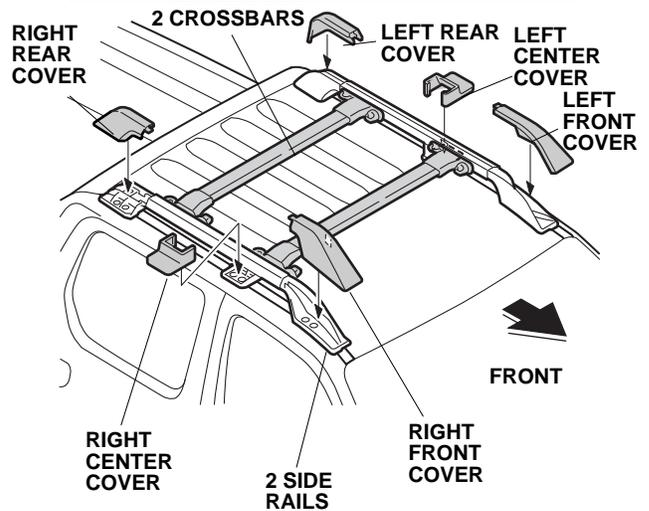
12. Loosen four thumb wheel screws on the crossbar holders. Align the marks on the crossbar holders with the marks on the side rails. Securely tighten the thumb wheel screws.
