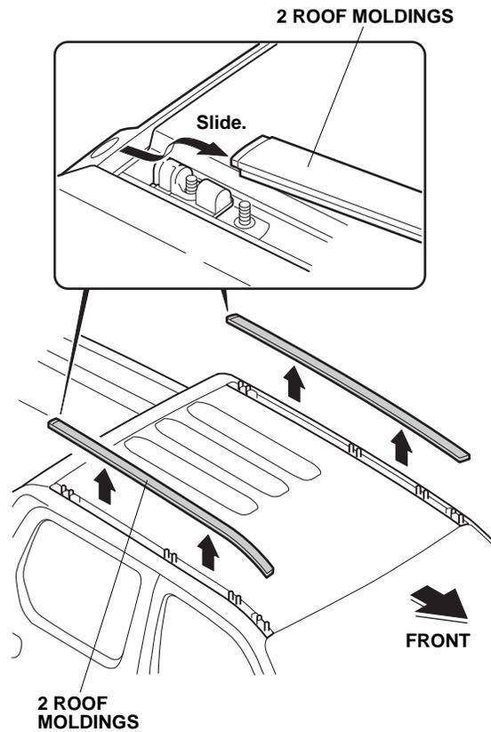
3. Using long nose pliers, remove the six clips from the roof channels. Discard the clips.
