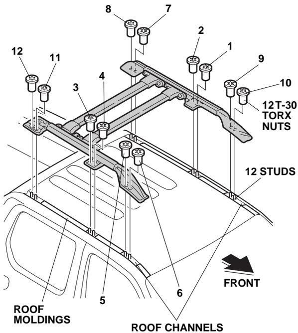
10. Install the roof rack to the roof channel with 12 T-30 Torx nuts. Torque the Torx nuts in the order shown to 10 N·m (7.4 lbf·ft).
