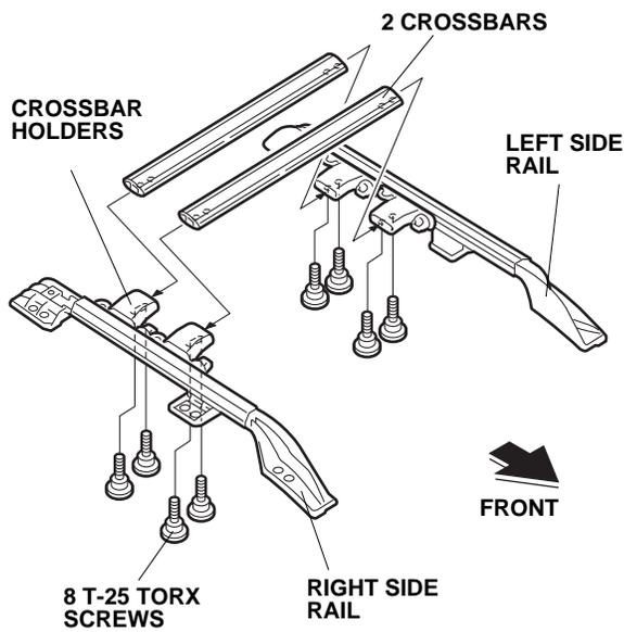
9. Align the holes in the left and right side rails with the 12 studs in the roof channel. Adjust the position of the roof moldings installed in step 5 if necessary.
