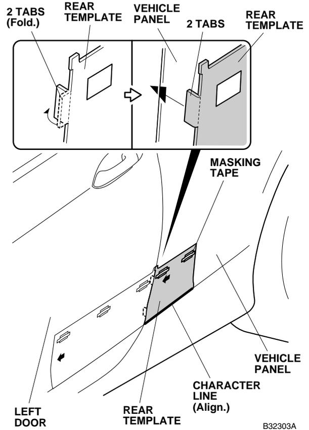
4. Insert the folded tabs of the rear template into the opening between the left door and the vehicle panel. Align the template with the character line, and tape the template to the door with strips of masking tape.
