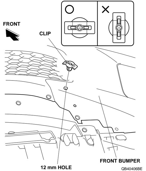
6. Using a pushpin, pierce the left front bumper at the two dimples on the front fenderwell.
