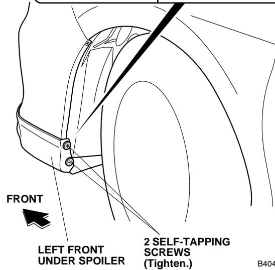
18. Turn the template over and repeat steps 2 through 17 to install the right front under spoiler on the right side of the vehicle.
