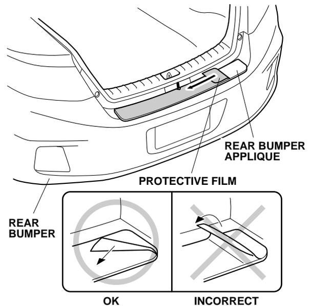
12. Repeat step 9 at the center of the lower section of the rear bumper applique.
