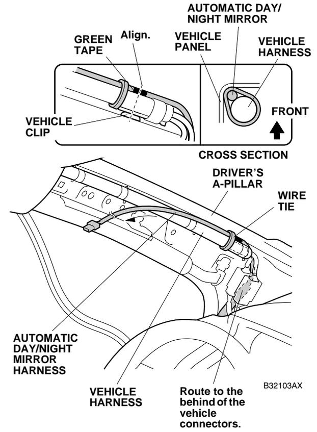
34. Route the automatic day/night mirror harness along the driver's A-pillar, and insert it under the headliner as shown. Be careful not to crease the headliner.
