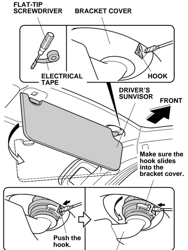
While pushing in on the hook, rotate the sunvisor backward about 45°. B32101BX
