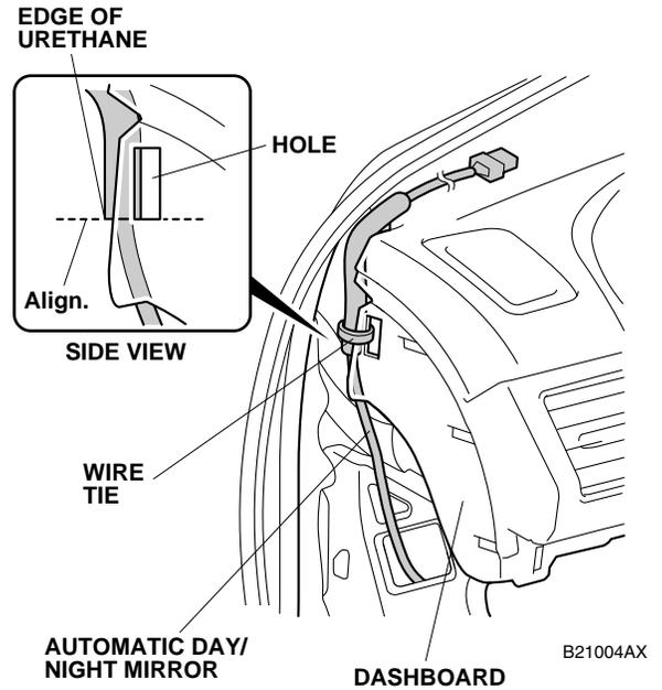
33. Route the automatic day/night mirror harness along the front of the vehicle harness. Align the green tape on the automatic day/night mirror harness with the vehicle clip, and secure the automatic day/night mirror harness to the vehicle harness with one wire tie.
