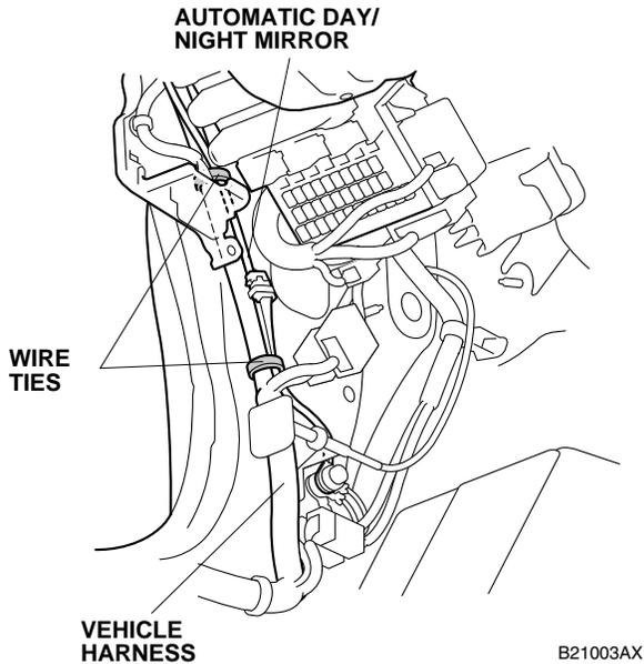
32. Route the automatic day/night mirror harness upward. Secure the automatic day/night mirror harness to the dashboard with one wire tie as shown.
