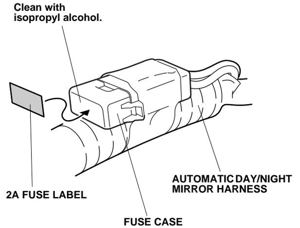
25. Attach the 2A fuse label to the fuse case on the automatic day/night mirror.
