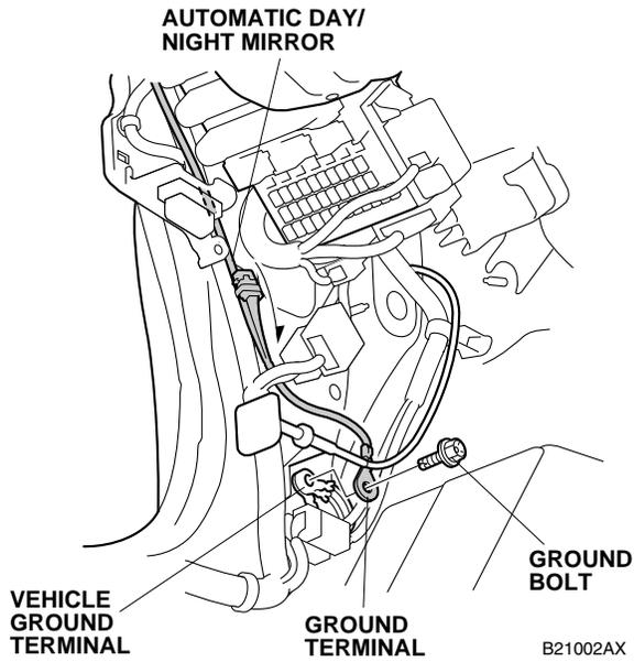
30. Remove the vehicle ground bolt. Secure the automatic day/night mirror harness ground terminal to the vehicle ground terminal, and reinstall the ground bolt.
