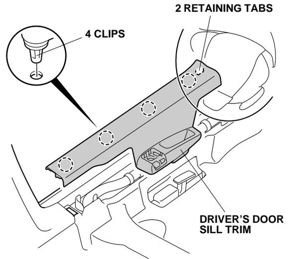
2-Door: Two retaining tabs and six clips.
