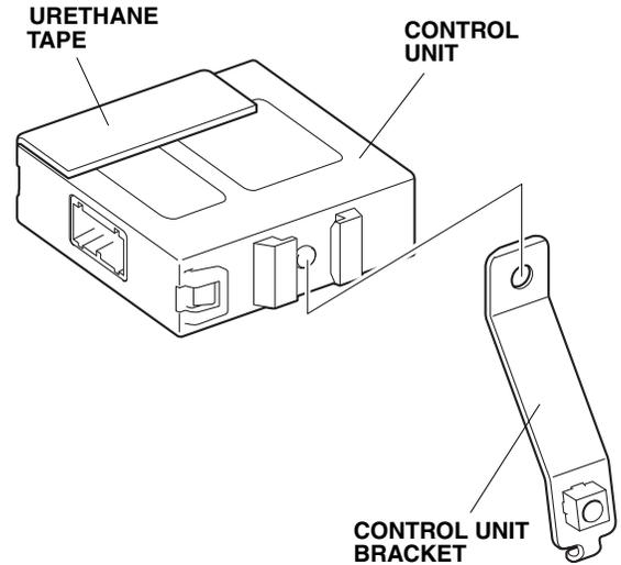
35. Using isopropyl alcohol on a shop towel, thoroughly clean the control unit where the urethane tape will attach. Attach the remaining piece of urethane tape (cut in step 33) to the control unit in the area shown.
