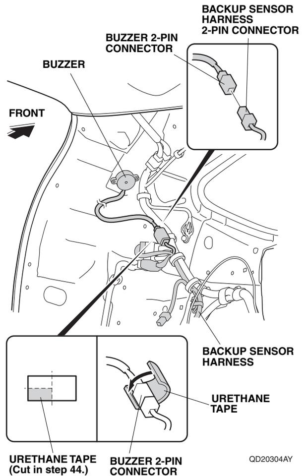
58. Attach the other piece of urethane tape (cut in step 44) around the buzzer 2-pin connector.
