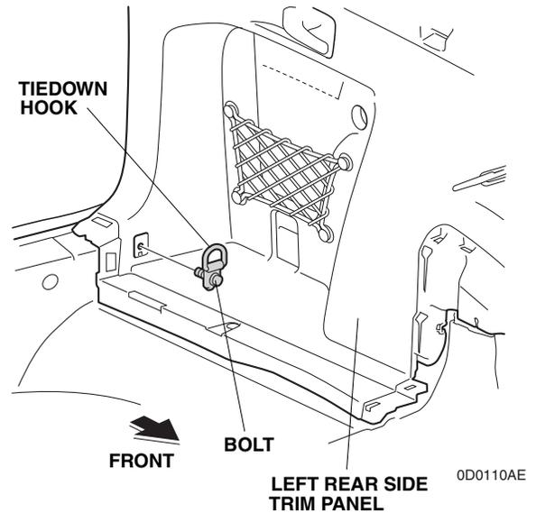
16. Pull away the weatherstrip from around the left rear side trim panel at the tailgate, and remove the door opening seal at the left rear door. Starting at the front, release the left rear side trim panel.
