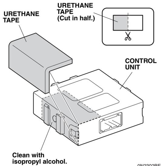
33. Using scissors, cut one urethane tape in half. Attach the cut piece of urethane tape to the control unit in the area shown.
