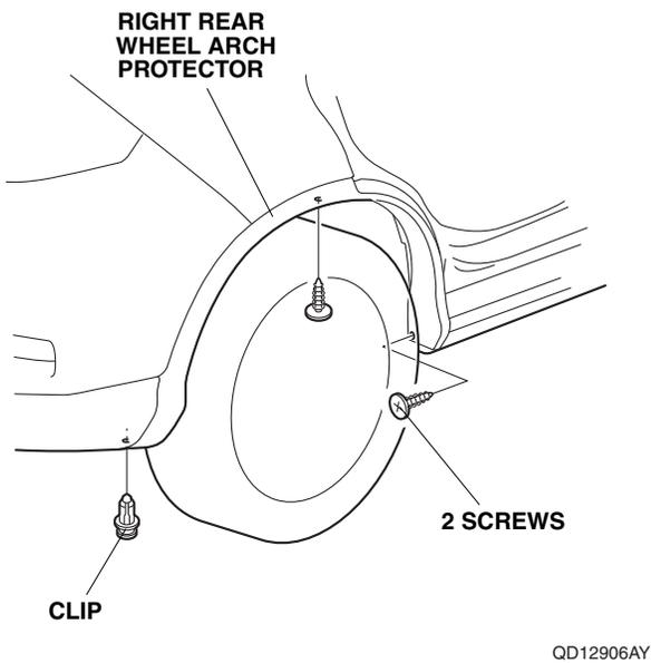
22. Remove the one clip and the two screws from the right rear wheel arch protector. If equipped, remove the splash guards.
