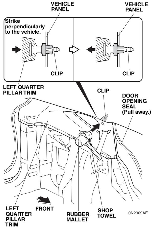
19. Using a rubber mallet wrapped with a shop towel, lightly tap the area marked "SIDE CURTAIN AIRBAG" on the left quarter pillar trim to push in the clip. Make sure to strike area perpendicularly to the vehicle.
