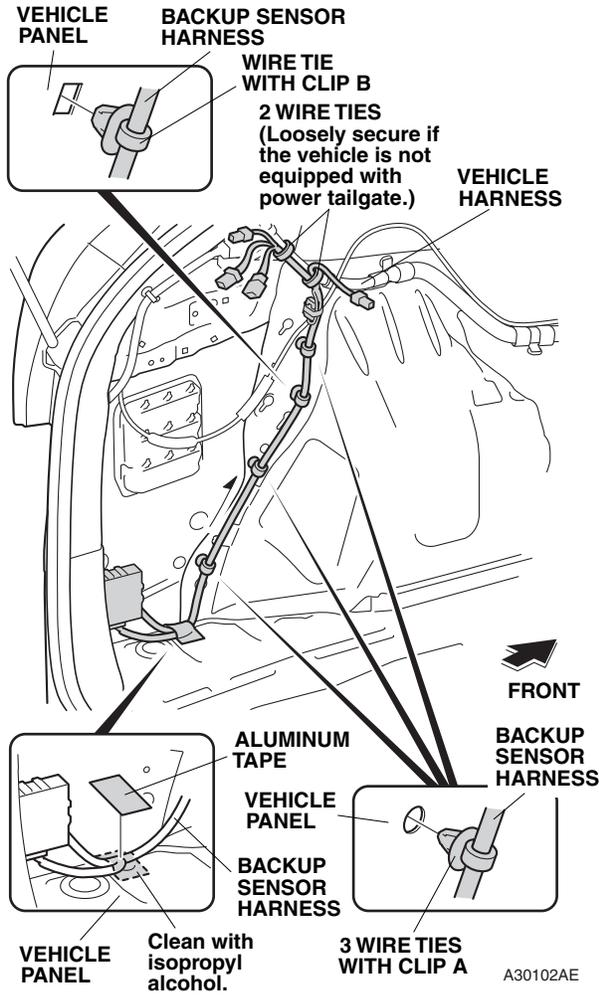
41. Route the backup sensor harness up along the vehicle harness, and secure it to the vehicle panel and vehicle harness with three wire ties with clip A, one wire tie with clip B, and two wire ties. If the vehicle is not equipped with the power tailgate, loosely secure the two wire ties.
