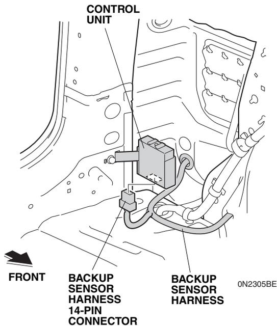
If the vehicle harness is installed in the area shown, continue with step 38; otherwise, go to step 40.
