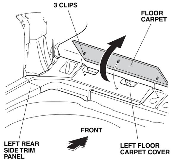
11. Remove the left floor carpet cover (three clips and two retaining tabs).
