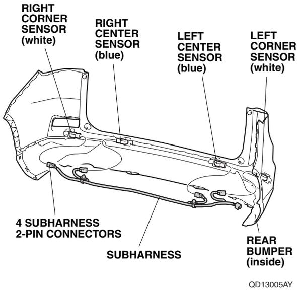
81. Secure the two subharness clips into two center sensor clips.
