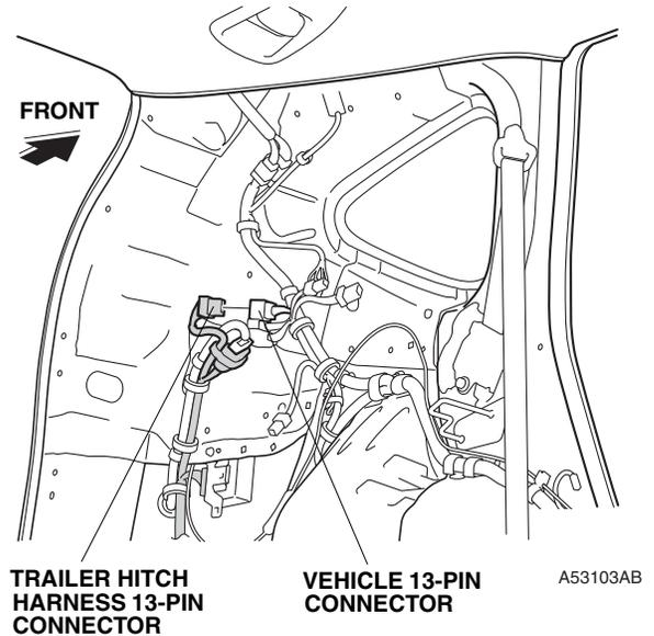
46. Plug the backup sensor harness 13-pin connector into the vehicle 13-pin connector.
