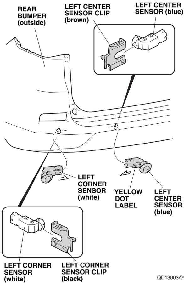
77. Secure the left corner sensor (white) and left center sensor (blue) with left corner sensor clip (black) and left center sensor clip (brown) as shown.
