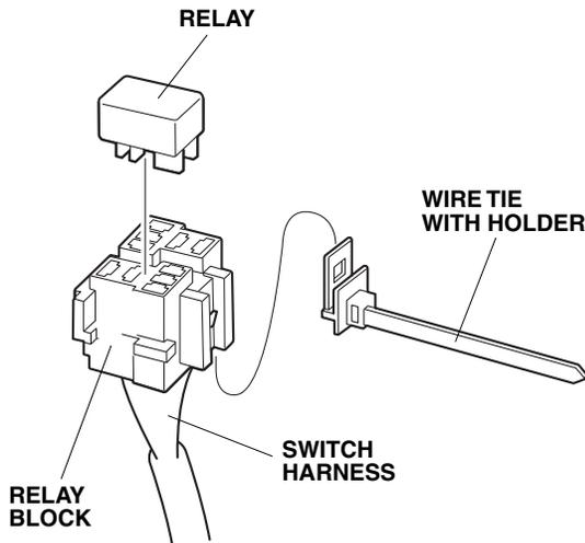
41. Install the one wire tie with holder into the switch harness relay block.
