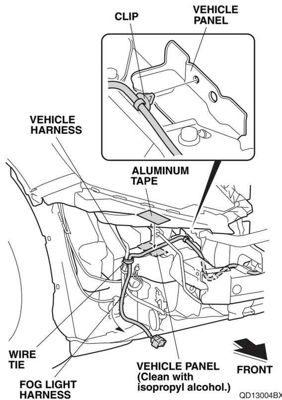
36. Using isopropyl alcohol on a shop towel, thoroughly clean the area where the aluminum tape will attach. Secure the fog light harness to the vehicle panel with one aluminum tape.
