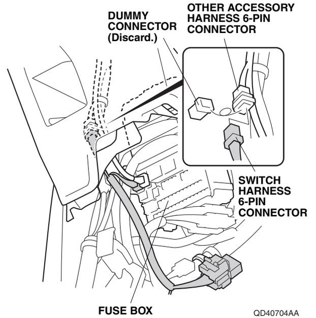
50. Plug the switch harness 6-pin connector to the other accessory harness 6-pin connector.
