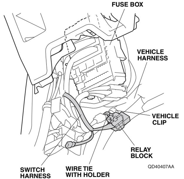
43. Plug the switch harness 1-pin connector to the vehicle 1-pin connector.
