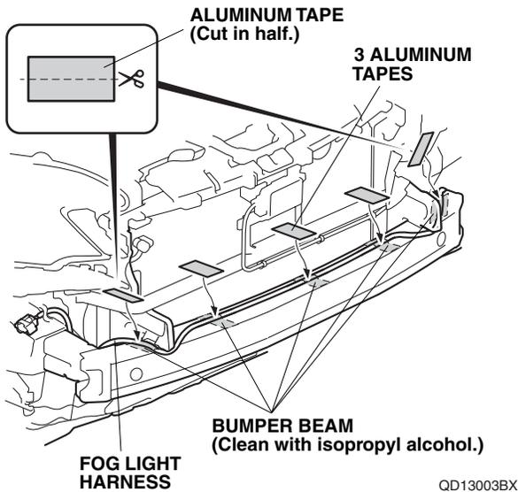
34. Using scissors, cut one aluminum tape in half. Secure the fog light harness to the bumper beam with two pieces of halved aluminum tape.
