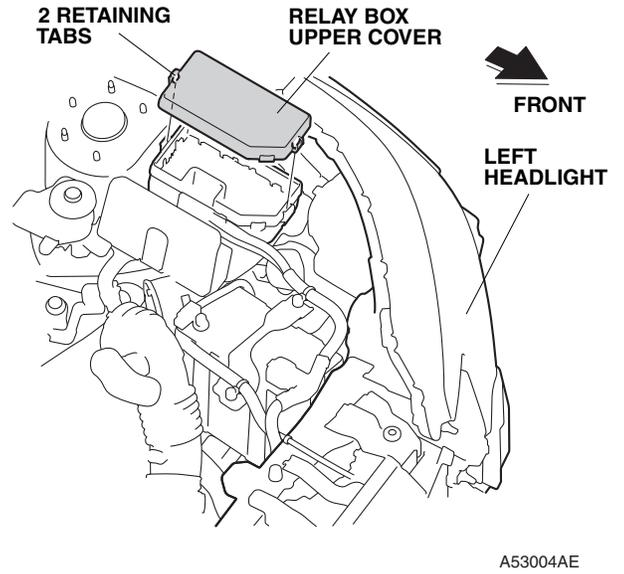
59. Using isopropyl alcohol on a shop towel, thoroughly clean the area where the fuse label will attach. Attach the fuse label to the relay box upper cover.
