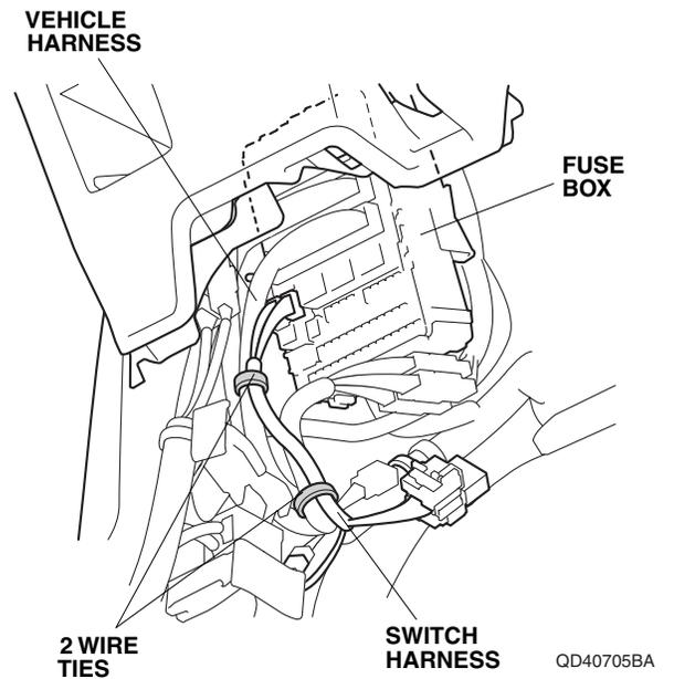
52. Unplug the vehicle connector from the light switch.
