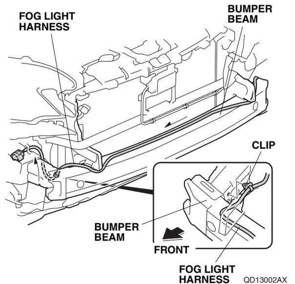
33. Using isopropyl alcohol on a shop towel, thoroughly clean the areas where the aluminum tapes will attach. Secure the fog light harness to the bumper beam with three aluminum tapes.
