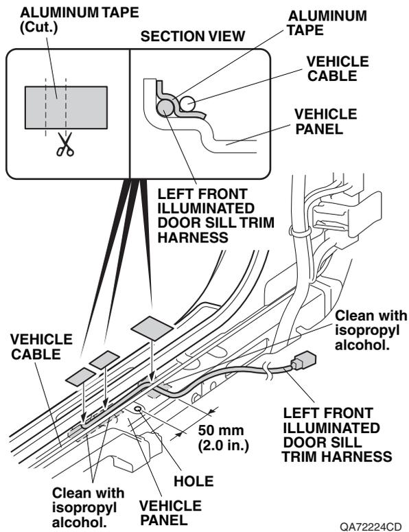
46. Using scissors, cut one aluminum tape, and secure the left front illuminated door sill trim harness to the vehicle panel with the three pieces of aluminum tape as shown.
