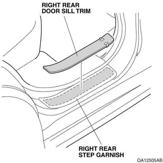
35. While applying light pressure against the right rear door sill trim, carefully remove the adhesive backings.
