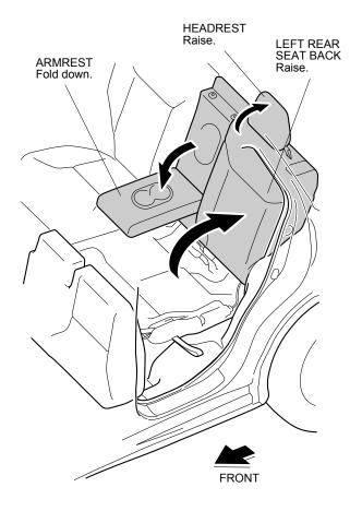
Install the left rear seat back cover over the left rear seat back. Insert the left rear seat back cover under the headrest guide, and insert the tab into the left rear seat back. Secure the fasteners to the left rear seat back.
