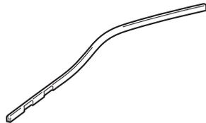
Seam sealant cutting tool
