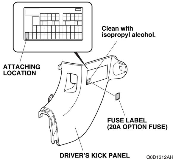
62. Attach the fuse label to the driver's kick panel.
