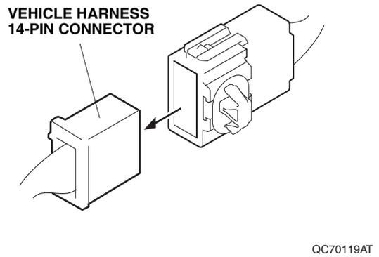
44. Release the retainer on the vehicle harness 14-pin connector. Connect the switch harness terminal into the vehicle harness 14-pin connector in the slot shown.
