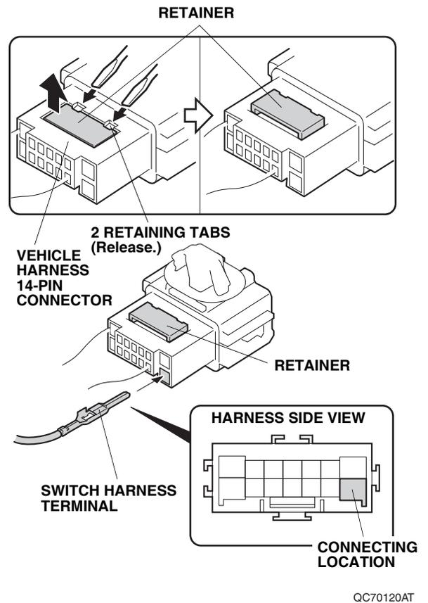
45. Replug the vehicle harness 14-pin connector and reinstall the 14-pin to its original position.
