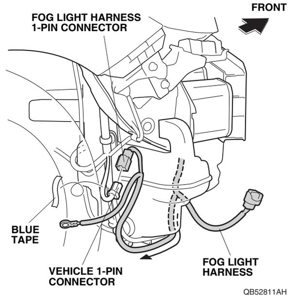
23. Plug the fog light harness 1-pin connector into the vehicle 1-pin connector as shown.
