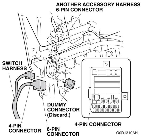
53. If the 4-pin connector is already used by another accessory, locate the 4-pin connector taped on another accessory harness. Plug the switch harness 4-pin connector into another accessory harness 4-pin connector.
