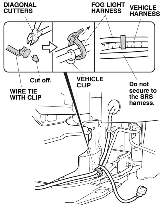
31. Secure the fog light harness to the vehicle harness with one wire tie with clip. Go to step 33.
