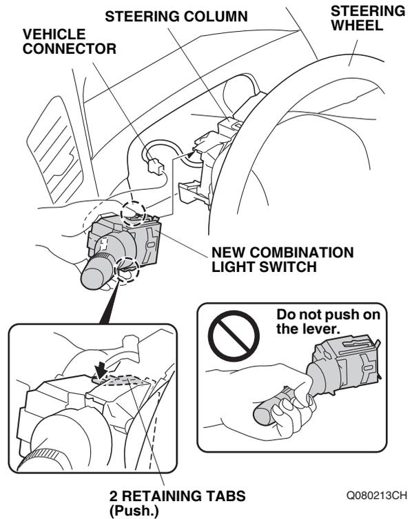
59. Plug the vehicle connector to the new combination light switch.
