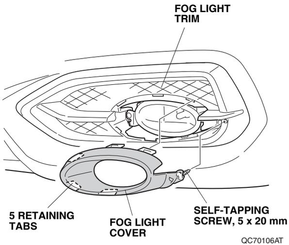
2. Remove the fog light (three self-tapping screws and unplug the vehicle connector).
