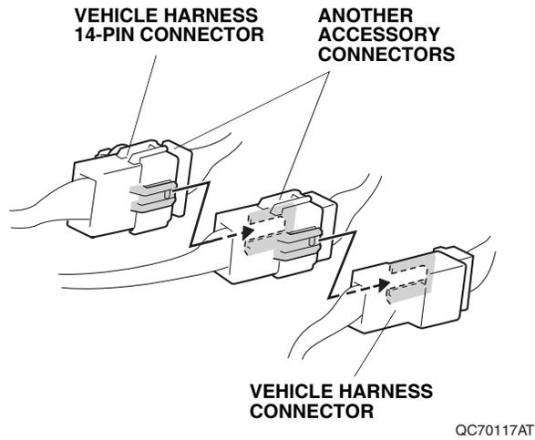
42. Remove the clip from the vehicle harness 14-pin connector, and install clip B on the vehicle harness 14-pin connector.
