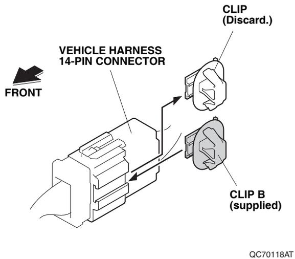
43. Unplug the vehicle harness 14-pin connector.
