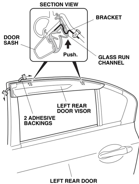
20. Using a soft towel, press and hold the left rear door visor against the door sash for 30 seconds.
