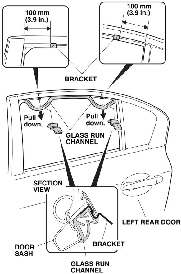
13. Install two brackets between the door sash and the glass run channel at the measurements shown. Seat the glass run channel properly around the brackets.
