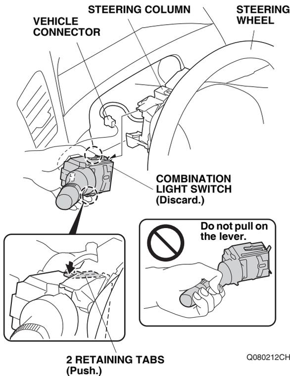
60. While pushing the two retaining tabs, slide the combination light switch out and remove it from the steering column.
