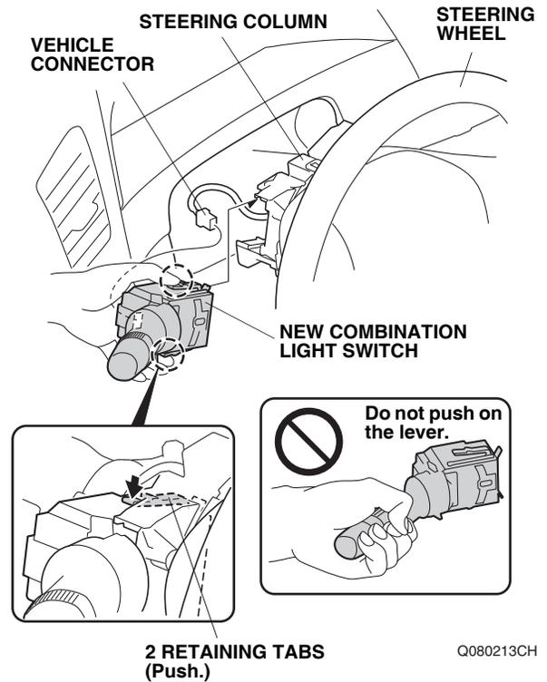
62. Plug the vehicle connector to the new combination light switch.
