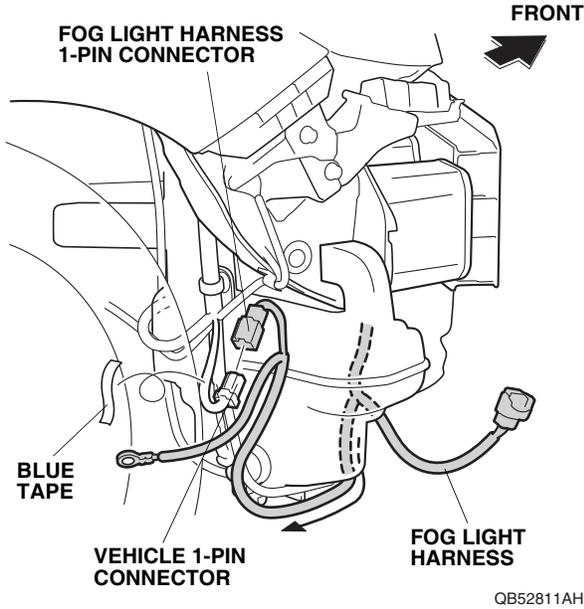
26. Plug the fog light harness 1-pin connector into the vehicle 1-pin connector as shown.
