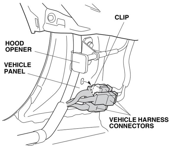
44. Remove the vehicle harness connectors from the vehicle harness 14-pin connector.
