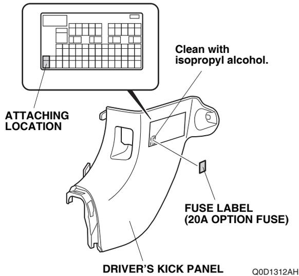
65. Attach the fuse label to the driver's kick panel.
