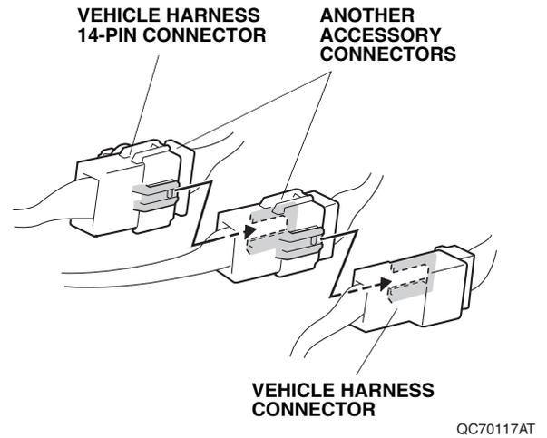
45. Remove the clip from the vehicle harness 14-pin connector, and install clip B on the vehicle harness 14-pin connector.
