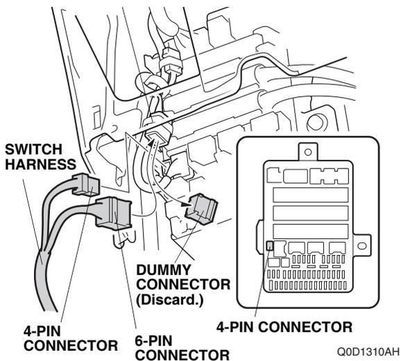
56. If the 4-pin connector is already used by another accessory, locate the 4-pin connector taped on another accessory harness. Plug the switch harness 4-pin connector into another accessory harness 4-pin connector.
