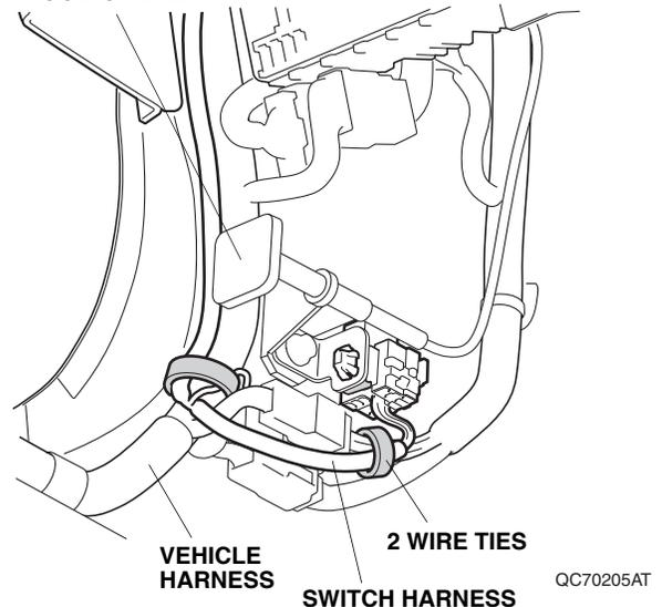
58. Secure the switch harness to the vehicle harness with two wire ties.
