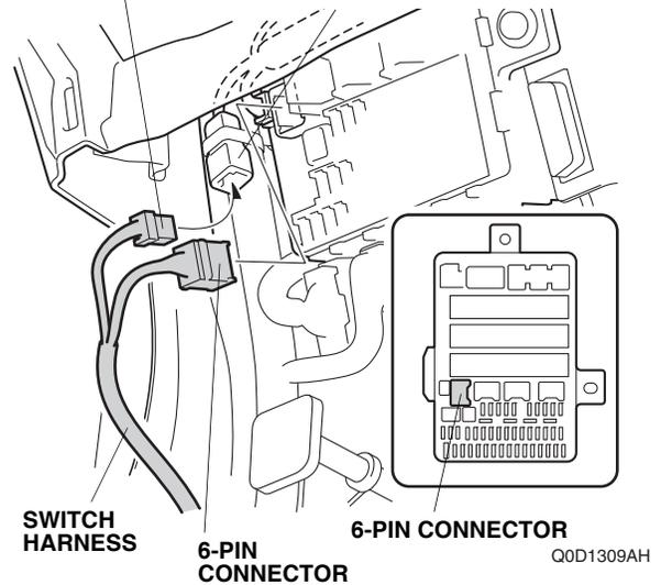
57. Secure the switch harness to the vehicle harness with two wire ties.
