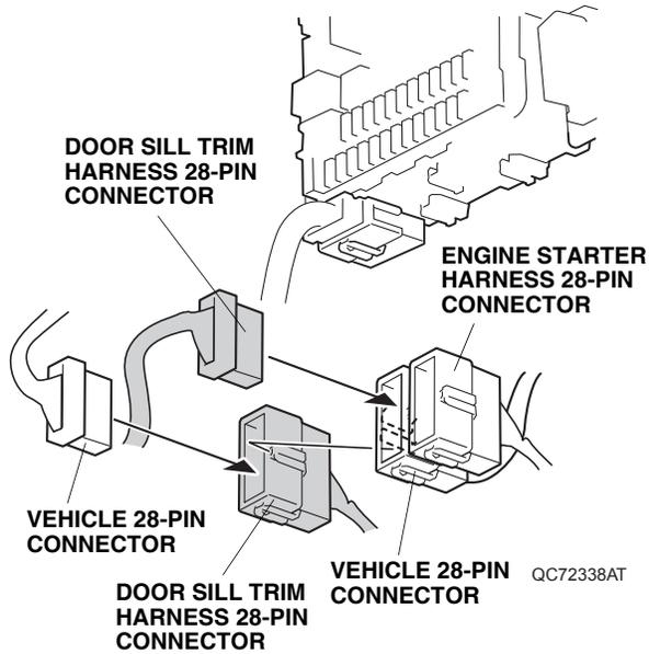
18. Plug the engine starter harness 28-pin connector into the engine starter harness 28-pin connector. Attach the connectors and clip on the engine starter harness as shown. Go to step 21.
