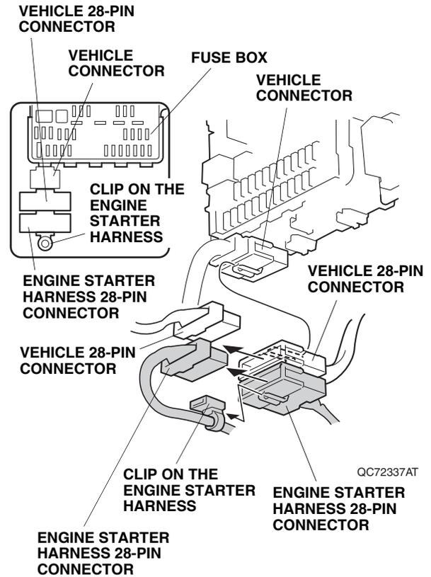
17. Plug the door sill trim harness 28-pin connector into the vehicle 28-pin connector. Plug the vehicle 28-pin connector into the remaining door sill trim harness 28-pin connector, and attach them to the vehicle 28-pin connector.
