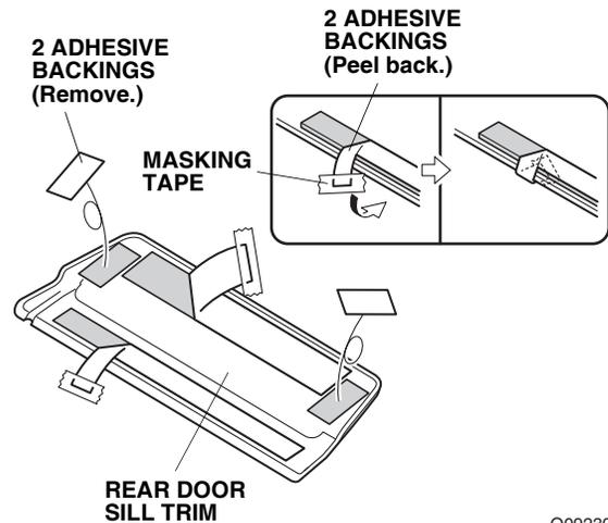
71. Position the rear door sill trim with the masking tape.
