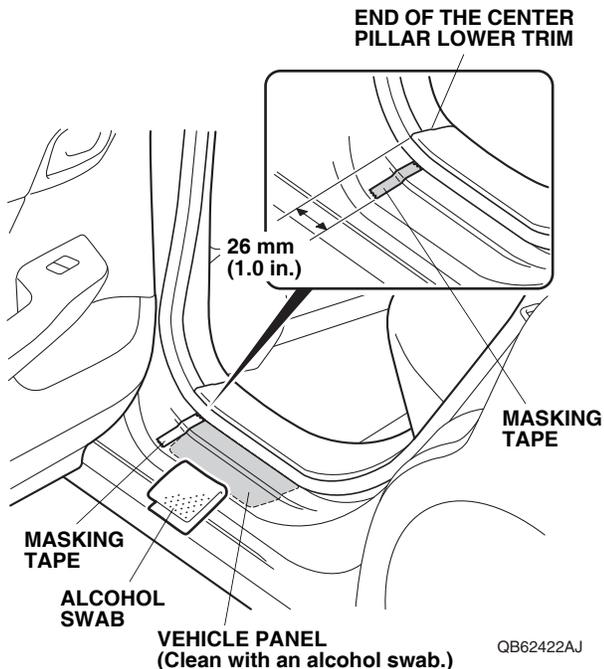
68. Attach a strip of masking tape to the vehicle panel at the measurement shown.
