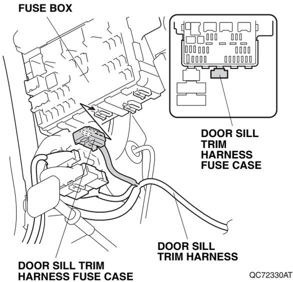
22. Secure the door sill trim harness to the vehicle harness with one wire tie.
