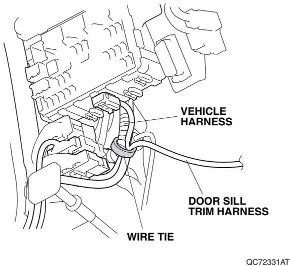
23. At the door sill area, secure the door sill trim harness to the vehicle harness with two wire ties.
