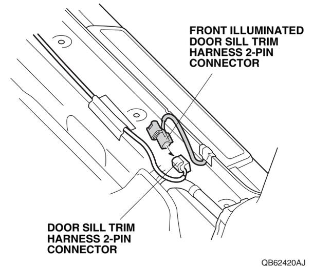
66. Bundle up the excess front illuminated door sill trim harness, and secure it to the vehicle harness with one wire tie with holder.
