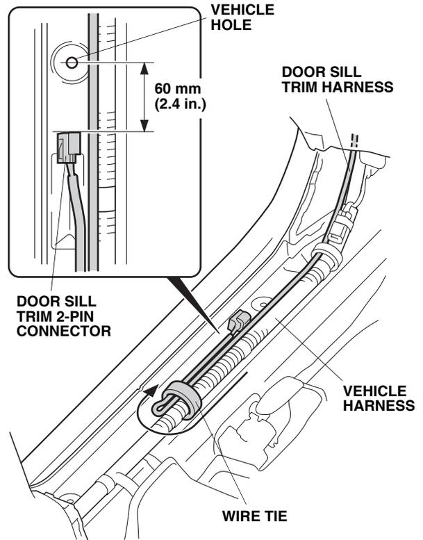
25. Route the other end of the door sill trim harness up and over to the vehicle harness. Secure the door sill trim harness to the vehicle harness with one wire tie.
