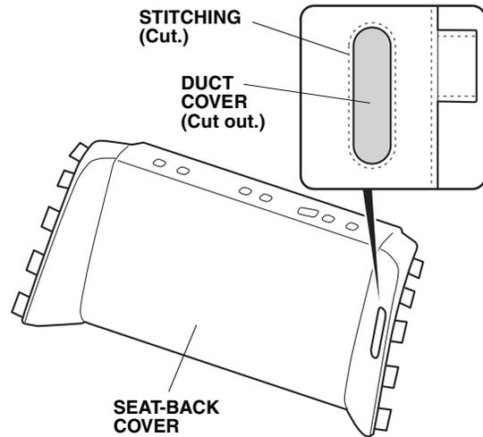
17. Pull out the center seat belt from the seat belt guide. Fit the seat-back cover onto the rear seat-back through the seat belts. Insert the seat-back cover under each headrest guide.
