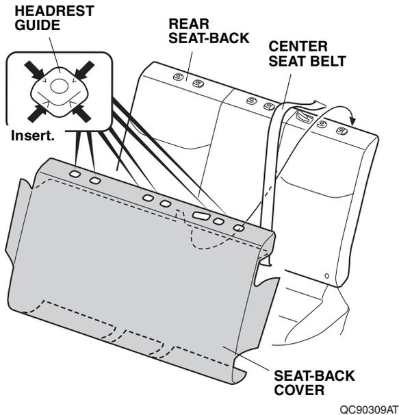
15. Secure the fasteners to the rear seat-back. Go to step 19.
