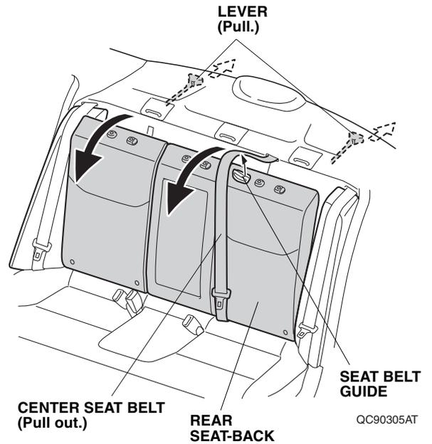
4. Open the trunk. Pull the lever, and fold the rear seat-back forward.
