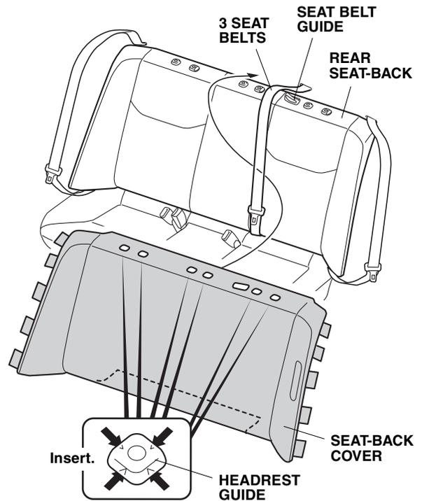
18. Insert the tabs to the rear seat-back. Secure the fasteners to the rear seat-back.
