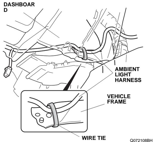
16. Inside the center lower panel opening, secure the ambient light harness to the vehicle harness with one wire tie.
