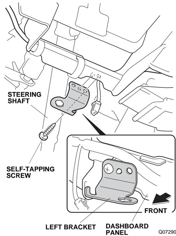
23. Install the ambient light to the left bracket by rotating it into position.
