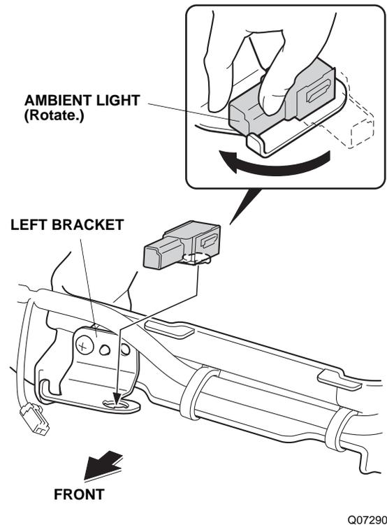
24. Plug the ambient light harness 2-pin connector into the ambient light.
