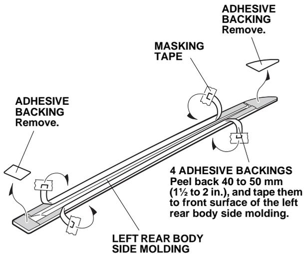
13. Align the edges of the left rear body side molding with the edges of the rear template, and install the left rear body side molding on the left rear door.
