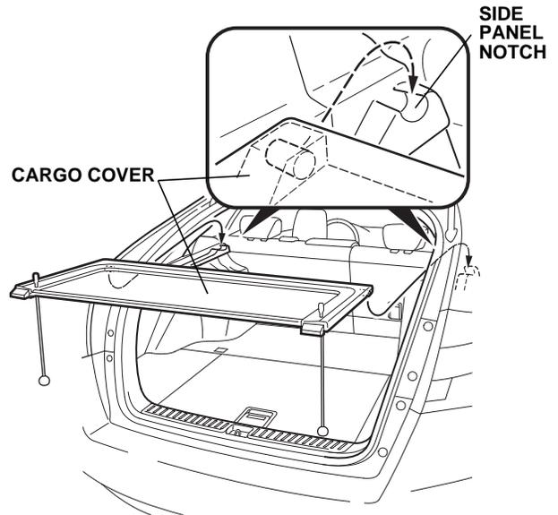
5. Install the cords onto the pins on the tailgate.
