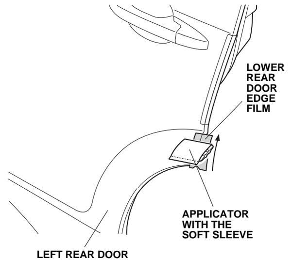
22. When you are satisfied that the lower door film is firmly attached to the edge of the door, slowly remove the outer protective film.
