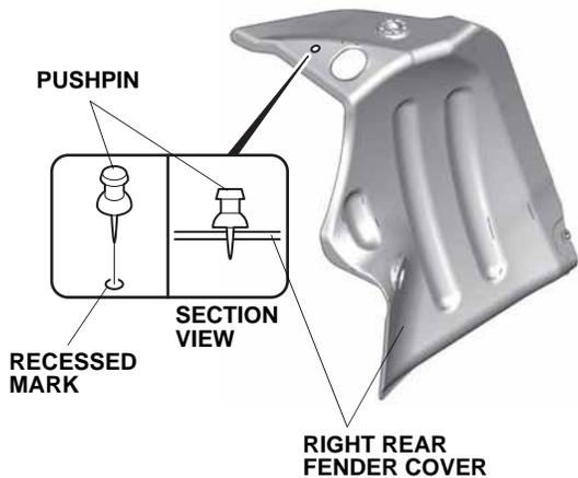
20. While wearing eye protection, drill the right rear fender cover at the pierced mark using a 3 mm drill bit first, then a 6 mm drill bit, 8 mm drill bit, and finish using a 10 mm drill bit.
