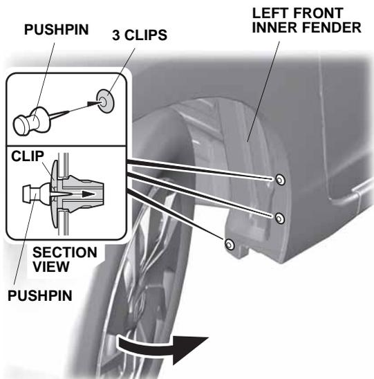
2. Using a pushpin, pierce the centers of the three clips on the left front inner fender.
