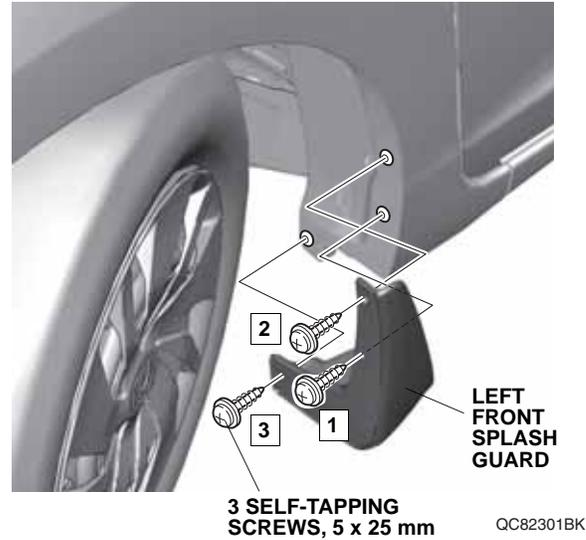
4. Turn the steering wheel clockwise, and repeat steps 2 and 3 to install the right front splash guard.
