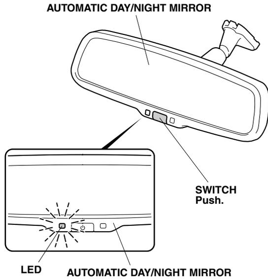
2. Push the switch. Check that the LED illuminates.
