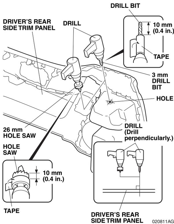
31. From inside of the driver's rear side trim panel, wear eye protection and drill one hole with a 3 mm drill bit.
