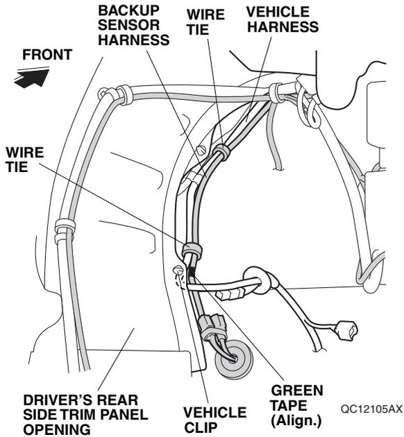
70. Secure the backup sensor harness to the vehicle harness with one wire tie.
