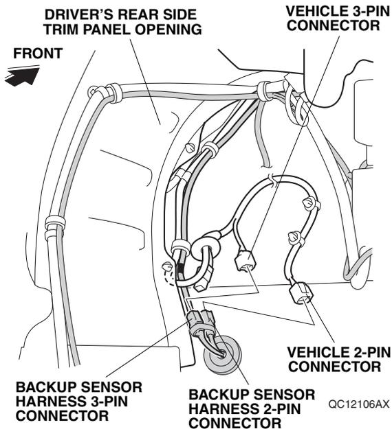
72. Plug the vehicle 2-pin connector to the backup sensor harness 2-pin connector.
