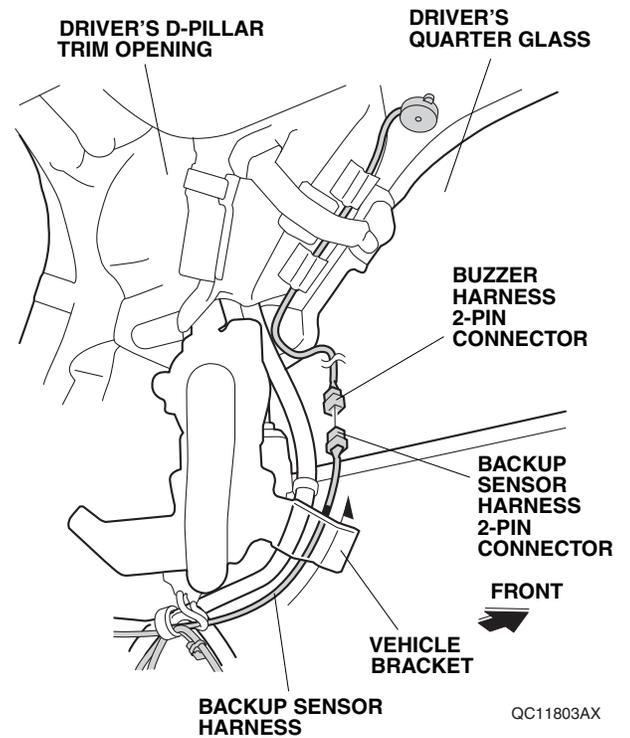
47. Plug the backup sensor harness 2-pin connector to the buzzer harness 2-pin connector.
