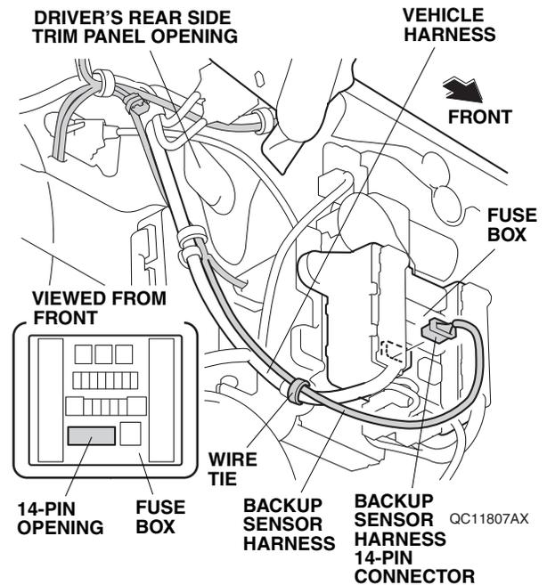
53. Secure the backup sensor harness to the vehicle harness with one wire tie. Go to step 56.
