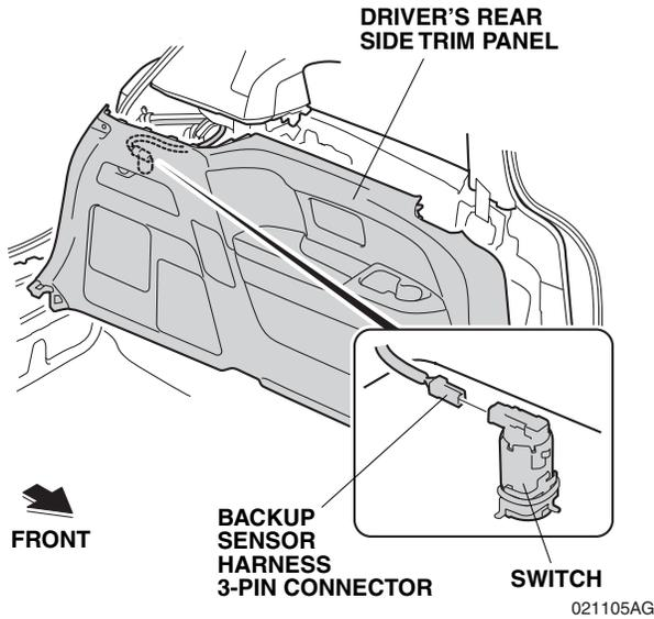
76. Bring the driver's rear side trim panel to the vehicle, and plug the backup sensor harness 3-pin connector to the switch.
