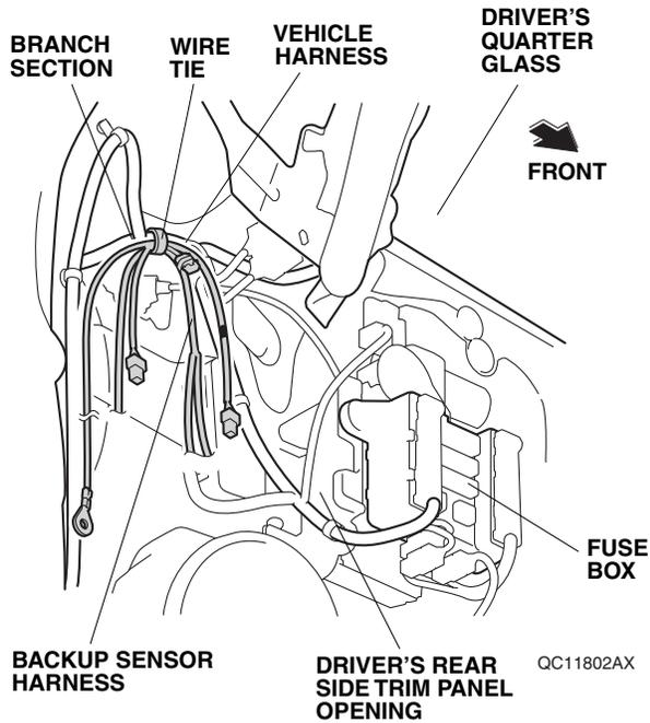
43. Route the backup sensor harness ground terminal along the vehicle harness.
