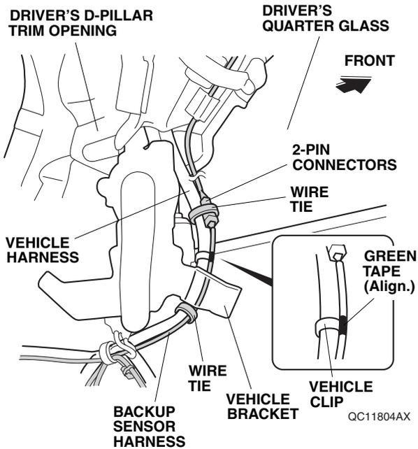
49. Secure the backup sensor harness to the vehicle harness with one wire tie.
