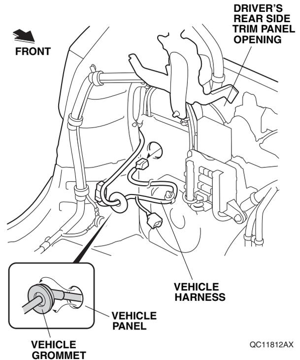
64. Route the backup sensor harness through the hole, and secure the grommet on the backup sensor harness to the vehicle panel as shown.
