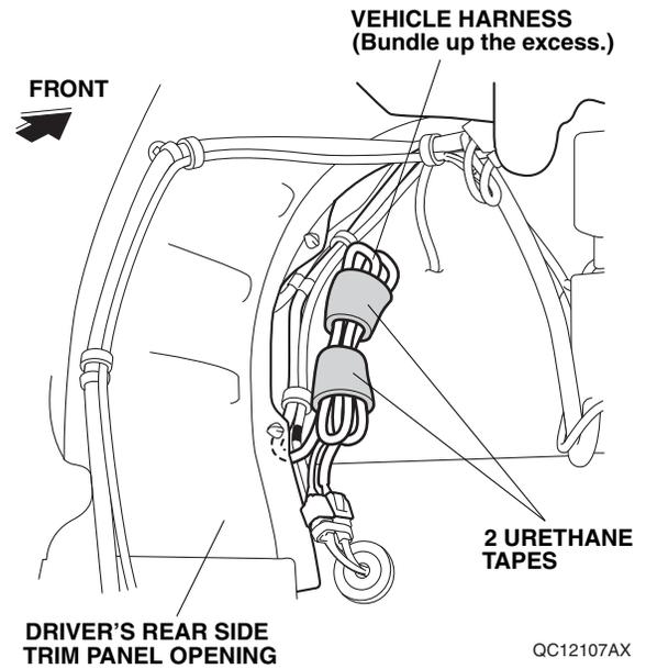
74. Secure the vehicle harness to the backup sensor harness and vehicle harness as shown.
