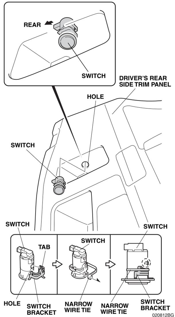
35. Align the tab on the switch bracket to the hole on the switch and secure the switch bracket to the switch with one narrow wire tie.
