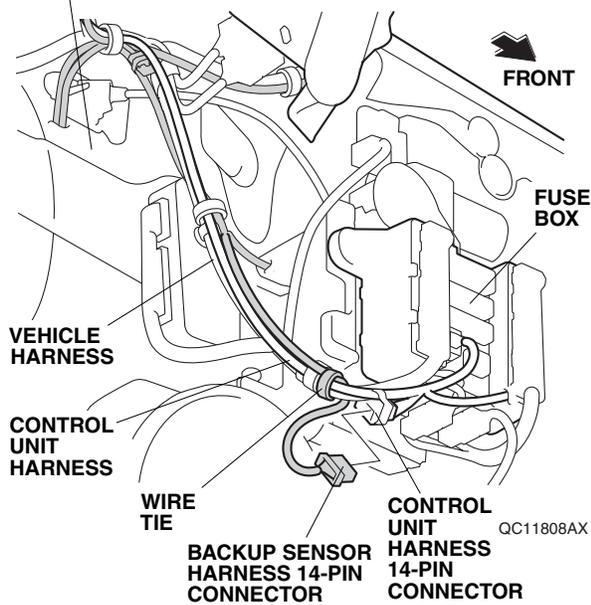
55. Secure the backup sensor harness to the vehicle harness and control unit harness with one wire tie.
