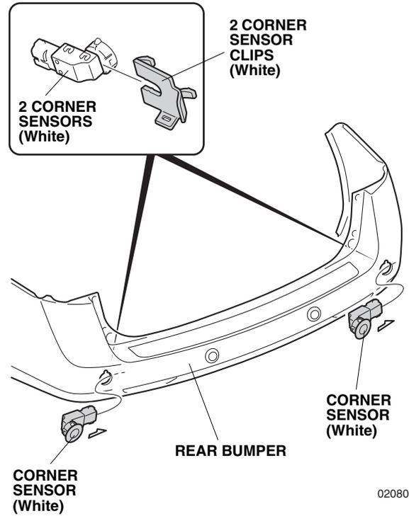
24. Secure two corner sensors (White) with two corner sensor clips (White) as shown.
