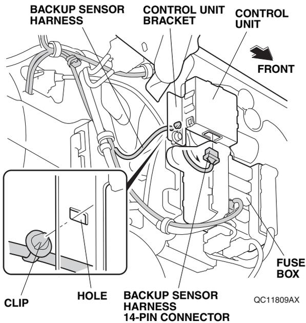
60. Secure the clip on the backup sensor harness to the hole on the control unit bracket as shown.
