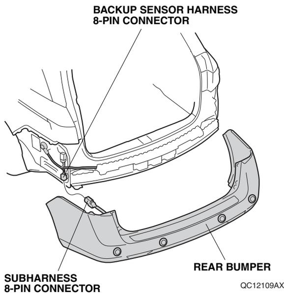
79. Check that all wire harnesses are routed properly and that all connectors are plugged in.
