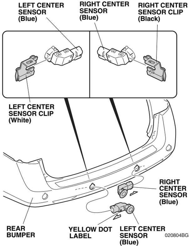
22. Secure the right center sensor (Blue) with right center sensor clip (Black) and the left center sensor (Blue) with left center sensor clip (White) as shown.
