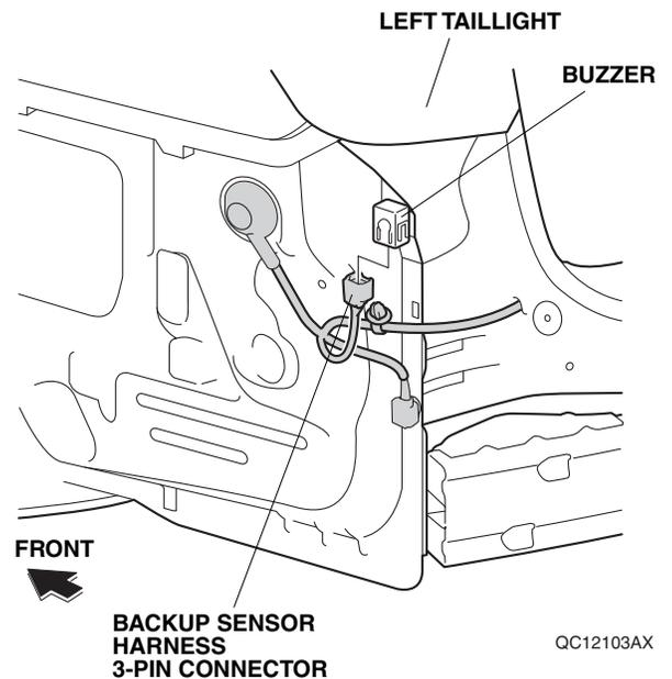
67. Route the backup sensor harness, and install the four clips on the backup sensor harness to the vehicle panel.
