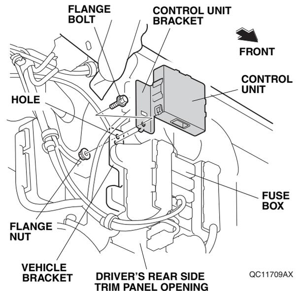
59. Route the backup sensor harness 14-pin connector, and plug it to the control unit.
