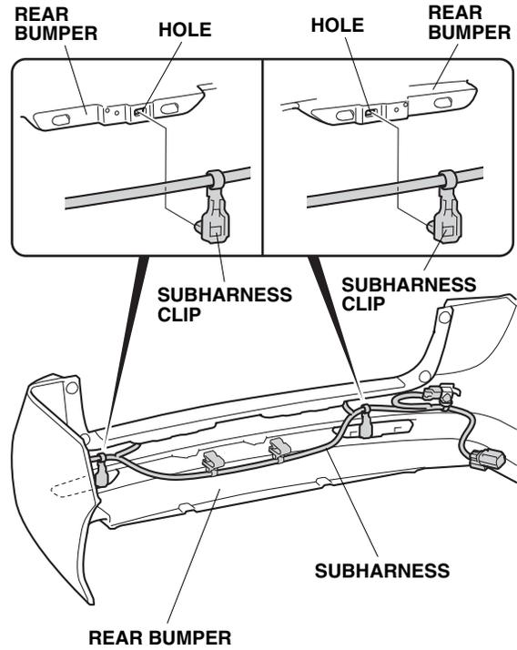
28. Secure two subharness clips to two ribs on the rear bumper as shown.
