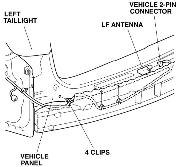
63. Release the vehicle grommet, pull out the vehicle harness from the inside of the vehicle.
