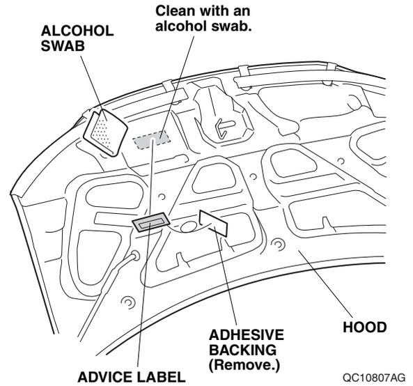
13. Remove the adhesive backing from the advice label, and attach the advice label to the hood as shown. NOTE: Do not attach the advice label over the other vehicle caution labels.
