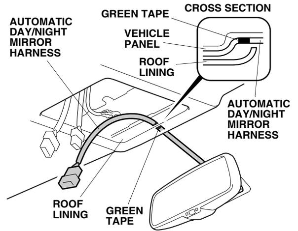
11. Locate the vehicle 6-pin connector and remove the blue tape. Plug the automatic day/night mirror harness 6-pin connector to the vehicle 6-pin connector.
