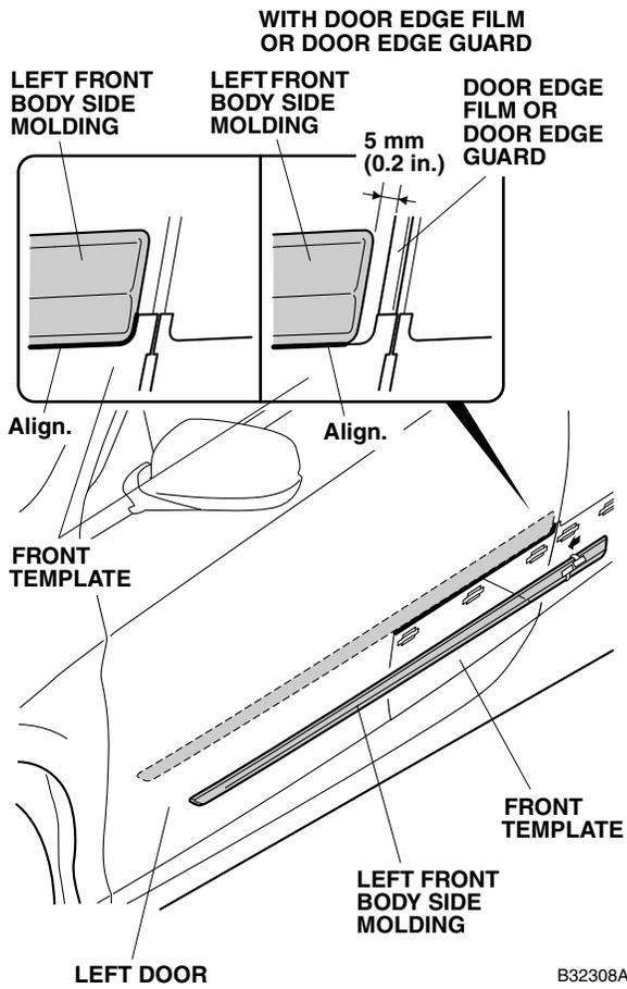
9. While applying light pressure against the left front body side molding, carefully remove the taped adhesive backings. Remove about 50 to 100 mm (2.0 to 4.0 in.) at a time.
