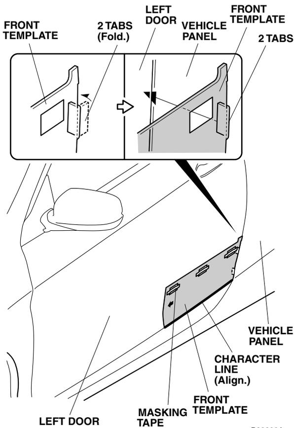
2. Insert the folded tabs of the front template into the opening between the left door and the vehicle panel. Align the template with the character line, and tape the template to the door with strips of masking tape.
