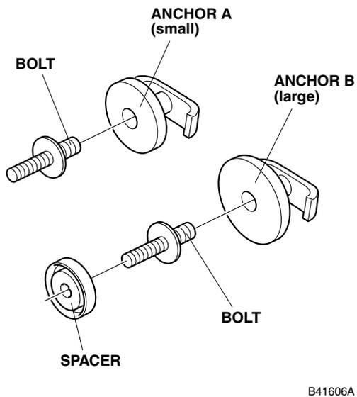
15. Install one spacer onto anchor B.
