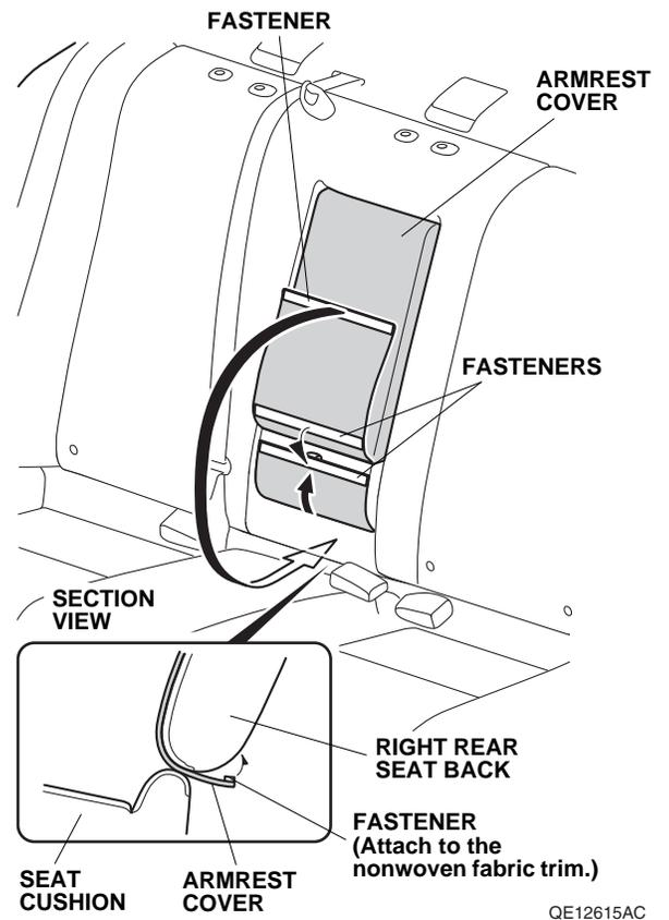
17. Insert the armrest cover between the right rear seat back and the rear seat cushion, secure the fastener to the right rear seat back.
