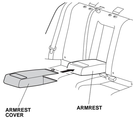
16. Raise the armrest. Pull out the armrest cover between the armrest and the right rear seat back, and secure the fasteners on the armrest cover as shown.
