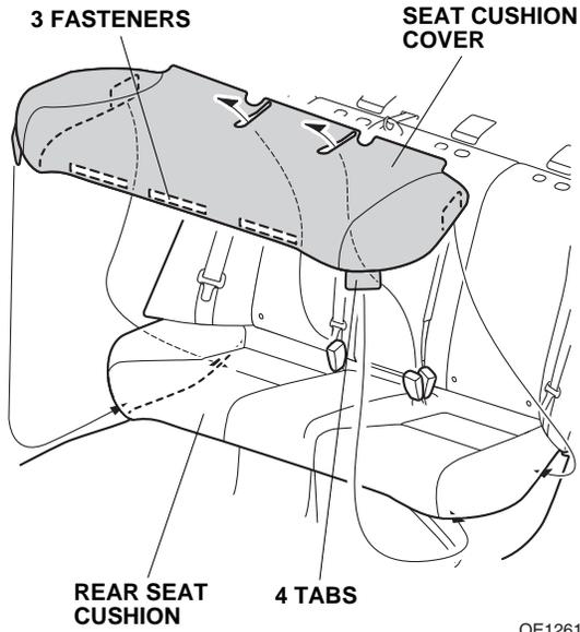
19. Insert the seat cushion cover between the rear seat back and the rear seat cushion, and secure the three fasteners to the rear seat cushion.
