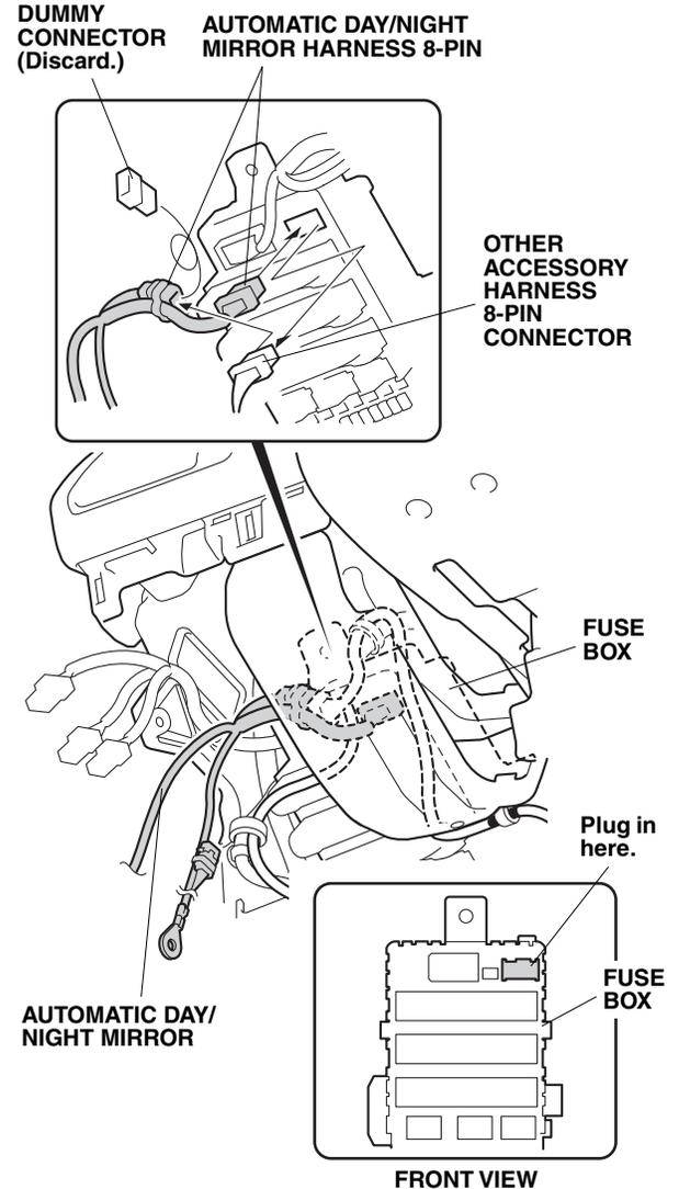
27. Route the automatic day/night mirror harness out of the square hole, and toward the outside of the vehicle as shown.
