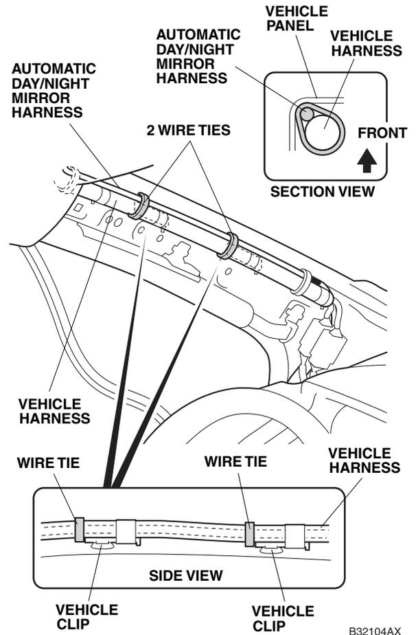
41. Check that all wire harnesses are routed properly and all connectors are plugged in.
