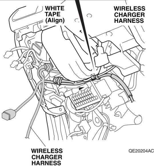
36. Attach the cut wire tie with clip around the white tape on the wireless charger harness and secure the wireless charger harness to the other accessory harness with one wire tie with clip.
