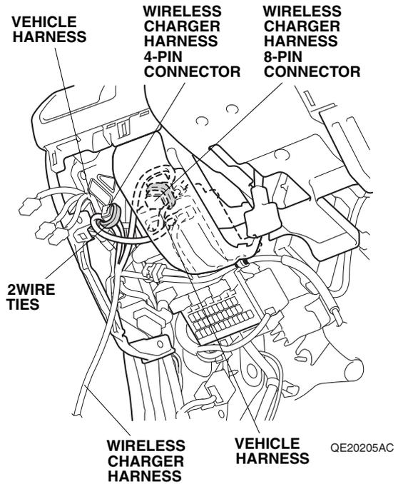
38. Remove the vehicle ground bolt and secure the wireless charger harness ground terminal to the vehicle ground terminals with one ground bolt. Do not put the ground terminal calkings on top of one another.
