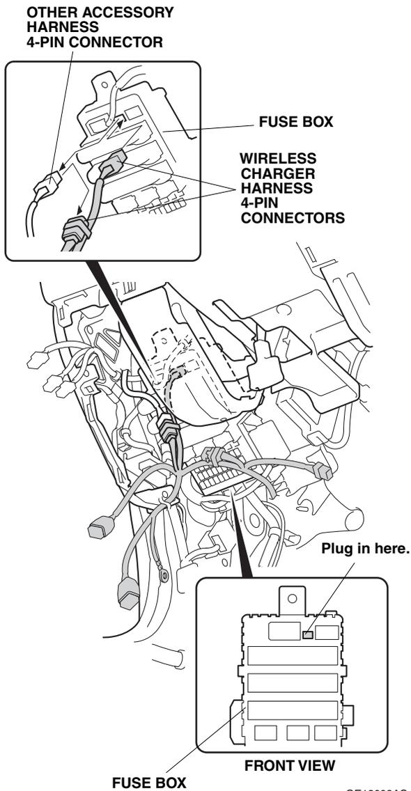
30. Plug the remaining wireless charger harness 4-pin connector into the fuse box.
