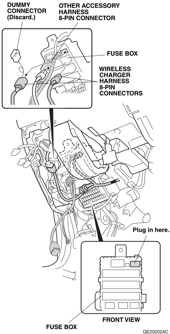
33. Plug the remaining wireless charger harness 8-pin connector into the fuse box.
