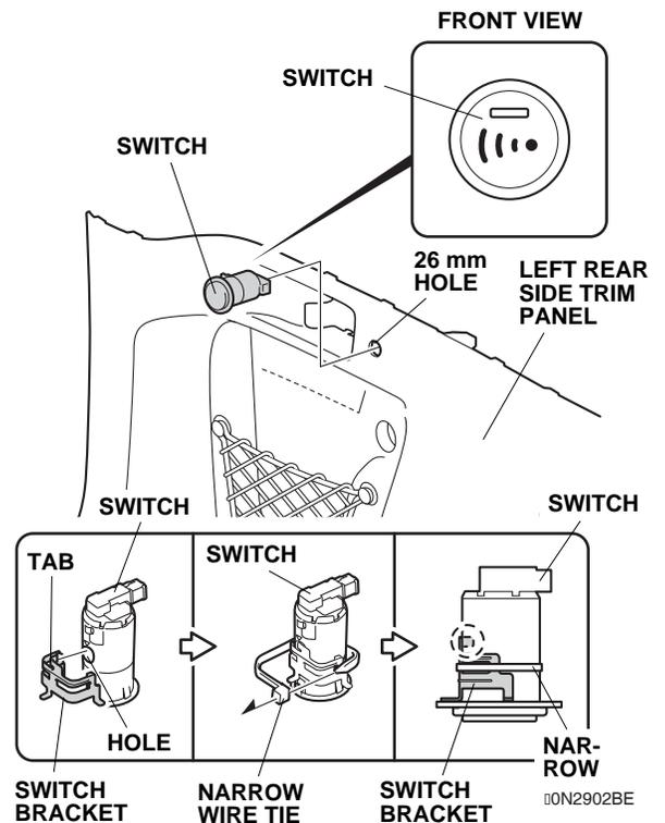
65. Align the tab on the switch bracket with the hole on the switch and secure the switch bracket to the switch with one narrow wire tie.
