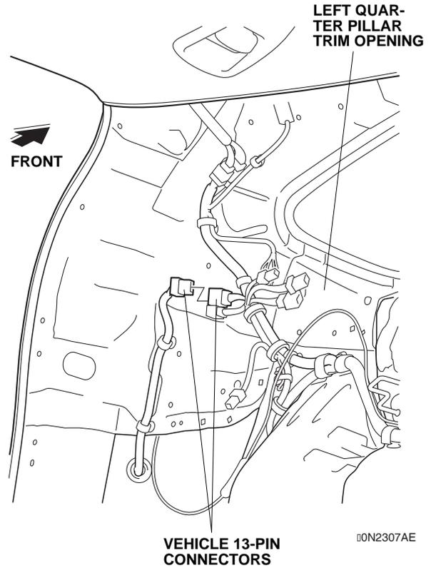
43. Slide the clip from the backup sensor harness 13-pin connector onto the vehicle connector clip.
