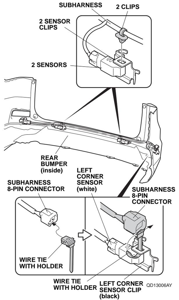
82. Install the wire tie with holder to the subharness 8-pin connector, and secure it to the left corner sensor clip (black) as shown.
