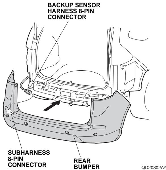
91. Check that all wire harnesses are routed properly and that all connectors are plugged in.
