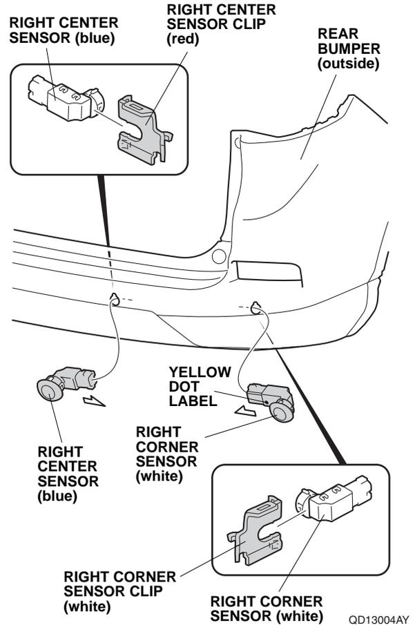
79. Secure the right corner sensor (white) and right center sensor (blue) with right corner sensor clip (white) and right center sensor clip (red) as shown.
