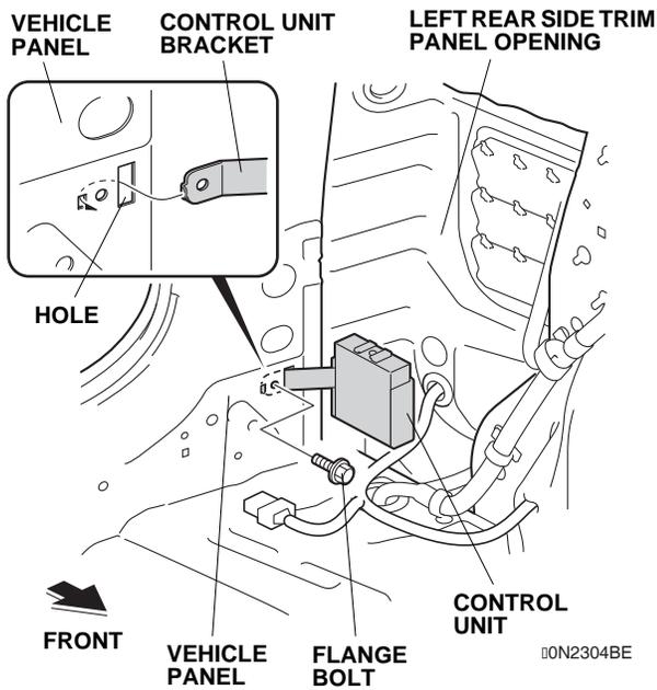
37. Plug the backup sensor harness 14-pin connector into the control unit.
