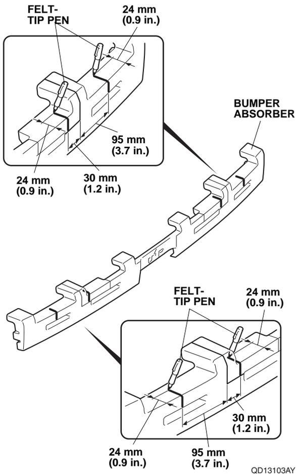
88. Using an utility knife, cut out the bumper absorber along the mark on each side of the bumper absorber.
