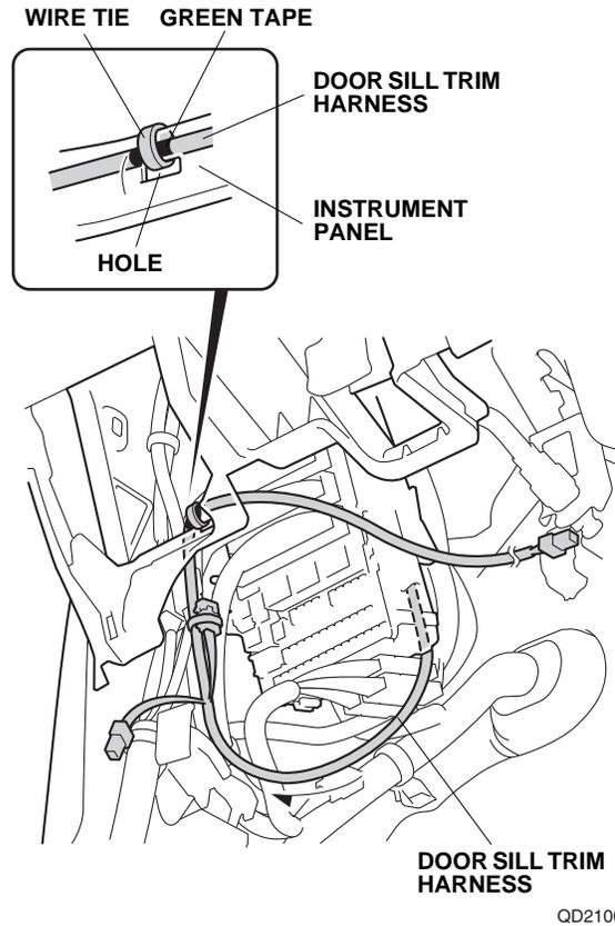
44. Secure the door sill trim harness to the vehicle harness with three wire ties.
