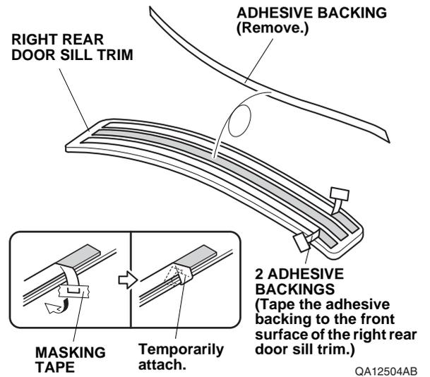
33. Using one alcohol swab, thoroughly clean the right rear step garnish where the right rear door sill trim will attach.
