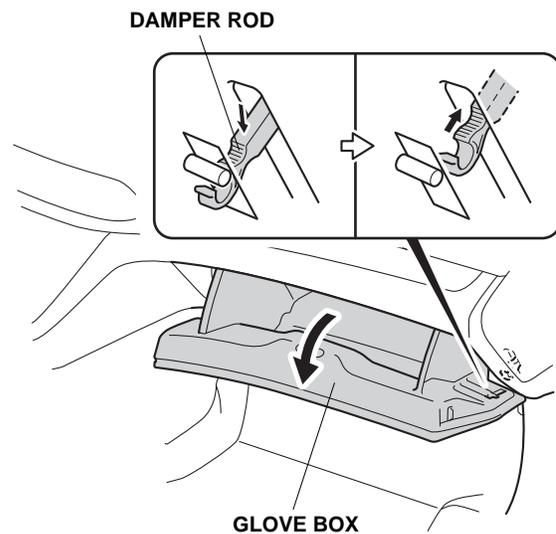
4. Close the glove box, and remove the two bolts from the glove box.
