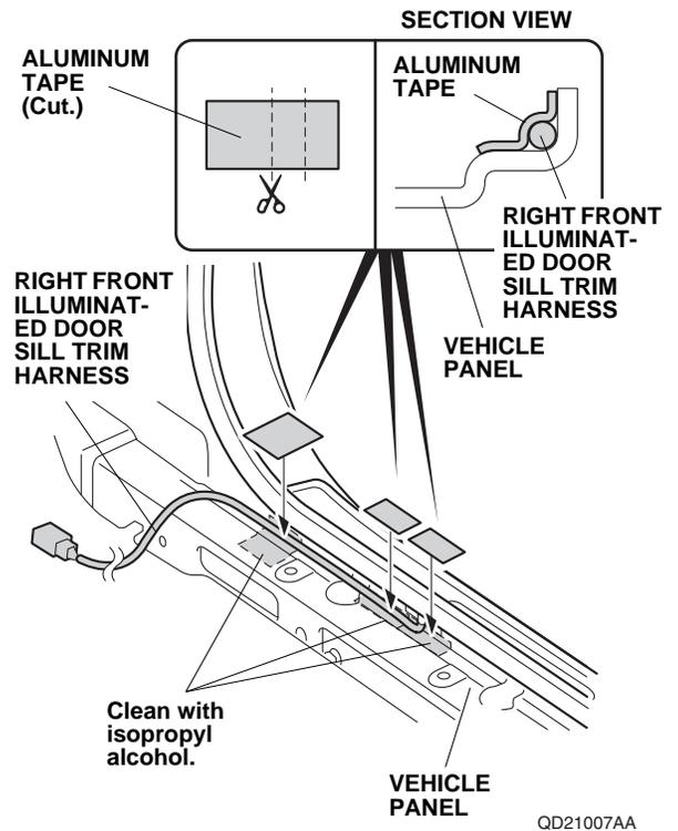
57. Using scissors, cut one aluminum tape, and secure the right front illuminated door sill trim harness to the vehicle panel with the three pieces of aluminum tape as shown.
