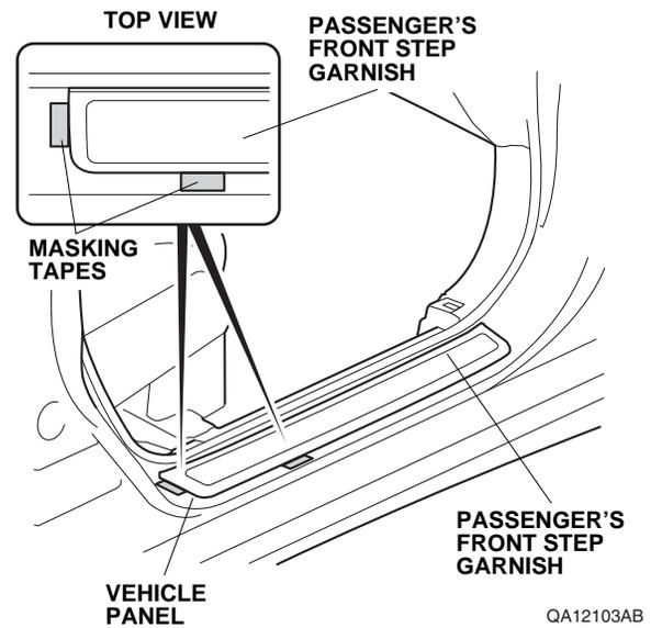
8. Pull away the door opening seal, and remove and discard the passenger's front step garnish.
