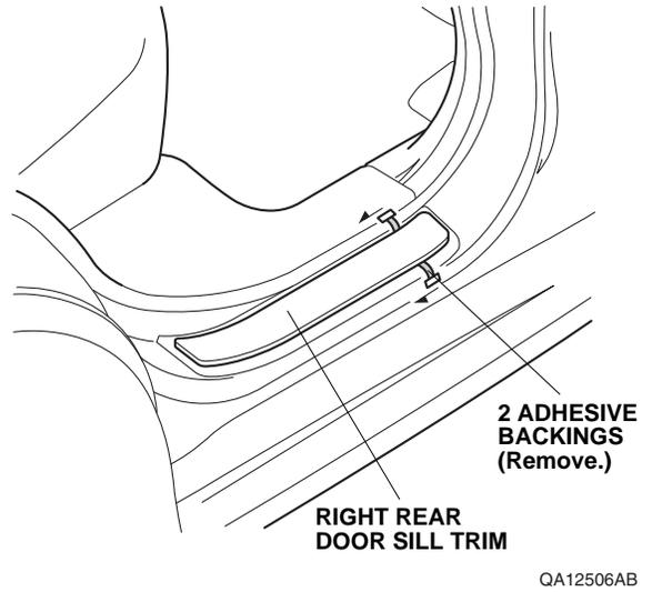
36. Repeat steps 19 through 35 to install the left front illuminated door sill trim and left rear door sill trim on the left side of the vehicle.
