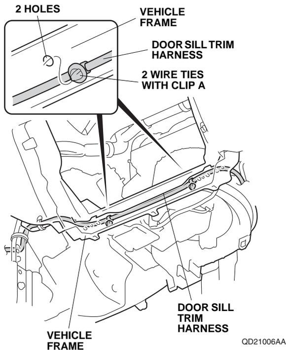
65. Check that all wire harnesses are routed properly and all connectors are plugged in.
