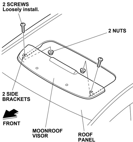
14. Position the moonroof visor with equal spacing on each side. Check that the rubber molding is not twisted or rolled under the visor.
