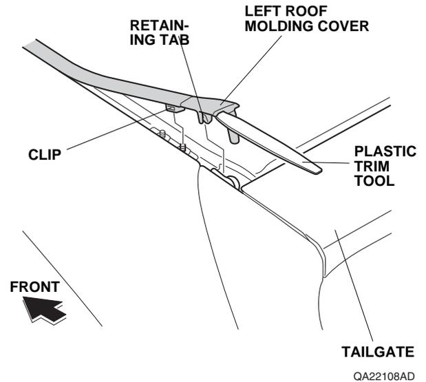
3. Pull the left roof molding toward the outside of vehicle to release the locking tab, and then press the locking tab toward the inside of vehicle, and release the left roof molding from the vehicle. When removing the left roof molding, start from the rear of vehicle and work towards the front.
