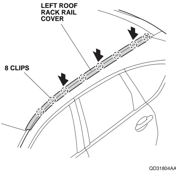
17. Secure the left roof rack rail cover to the left roof rack base with one self-tapping screw.
