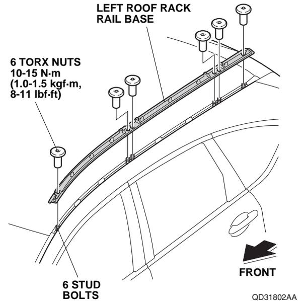
15. Hook the front of the left roof rack rail cover to the left roof rack base.
