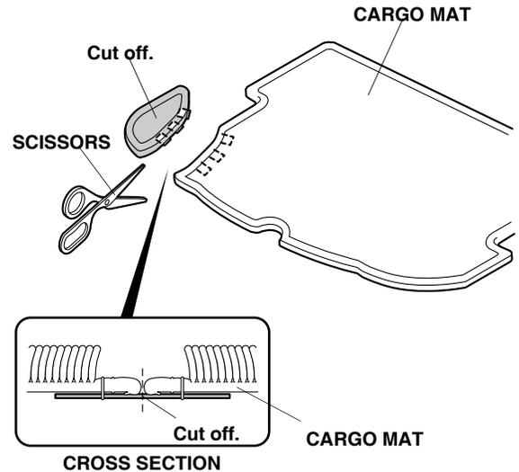
2. Open the hatch, and place the cargo mat on the cargo floor as shown.
