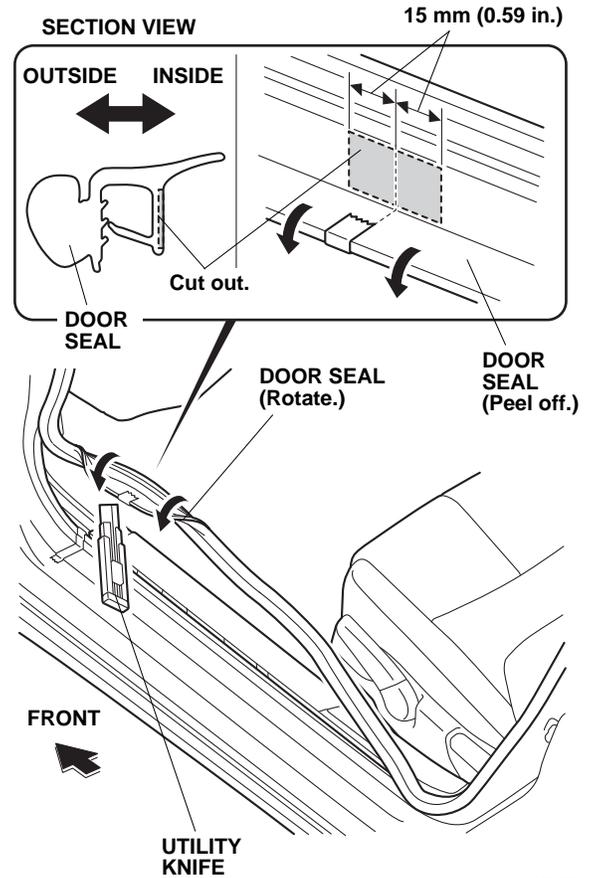
16. Using a utility knife, make a slit in the door seal at the location shown to expose the small metal plates.
