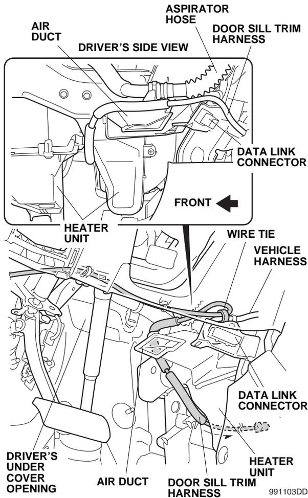
44. Secure the door sill trim harness to the vehicle harness with one wire tie.
