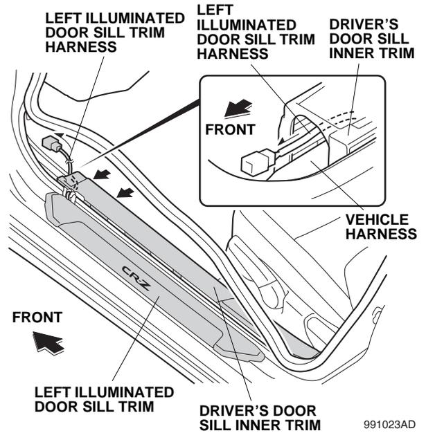
32. Install the driver's door sill inner trim and door seal.
