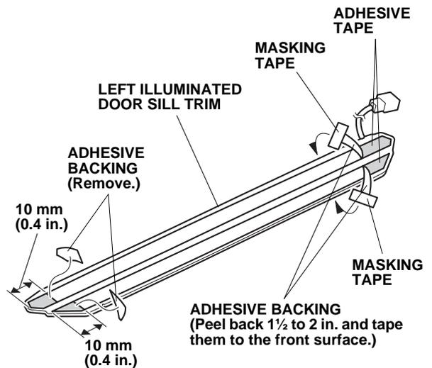
23. Using one alcohol swab, thoroughly clean the area where the left illuminated door sill trim will attach.
