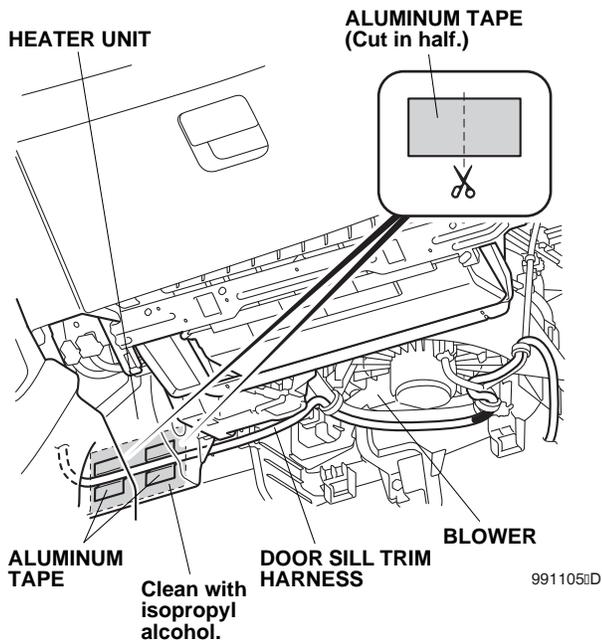
49. Using scissors, cut one aluminum tape in half. Secure the door sill trim harness to the back of the heater unit with two halves of aluminum tape as shown.
