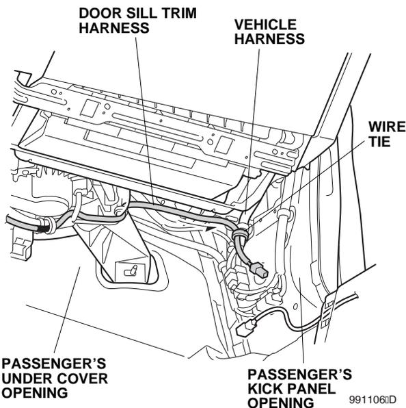
51. Secure the door sill trim harness to the vehicle harness with one wire tie.
