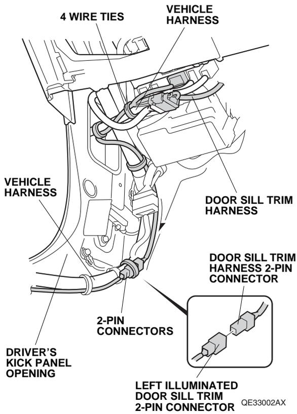
39. Secure the door sill trim harness and 2-pin connectors to the vehicle harness with four wire ties.
