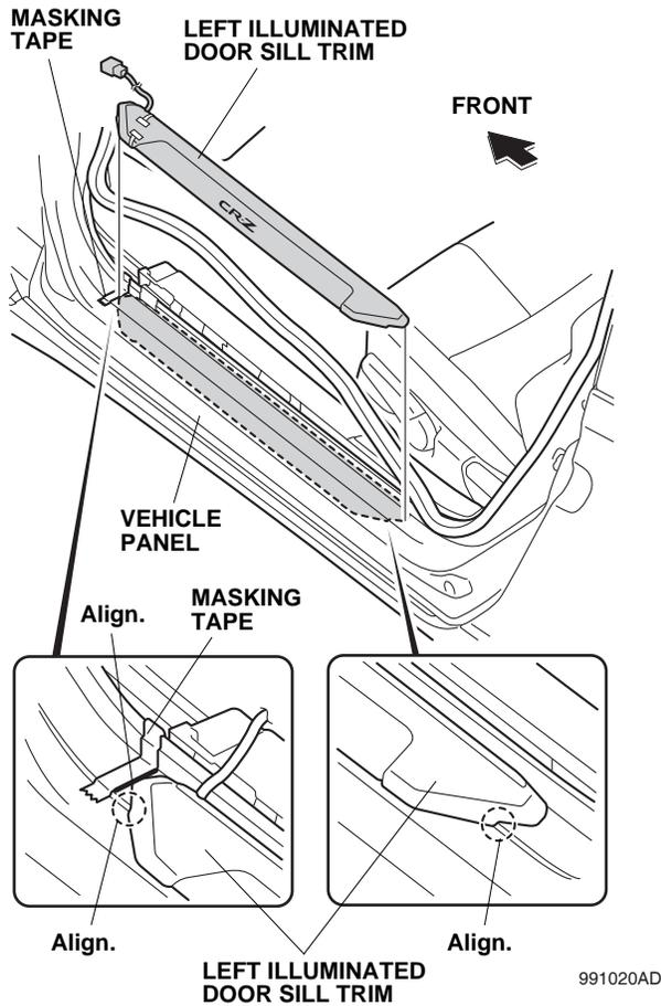
25. While applying light pressure against the left illuminated door sill trim, carefully remove the adhesive backings.
