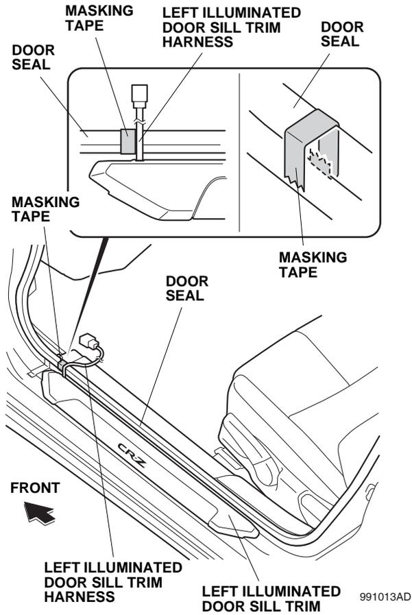
12. Route the left illuminated door sill trim harness over the door seal. Apply masking tape to the door seal to mark where the illuminated door sill trim harness crosses the door seal.
