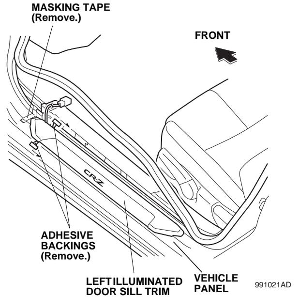
26. Using the palm of your hand, firmly press the left illuminated door sill trim against the vehicle panel.
