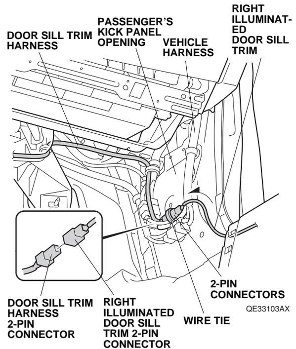
53. Secure the 2-pin connectors to the vehicle harness with one wire tie.
