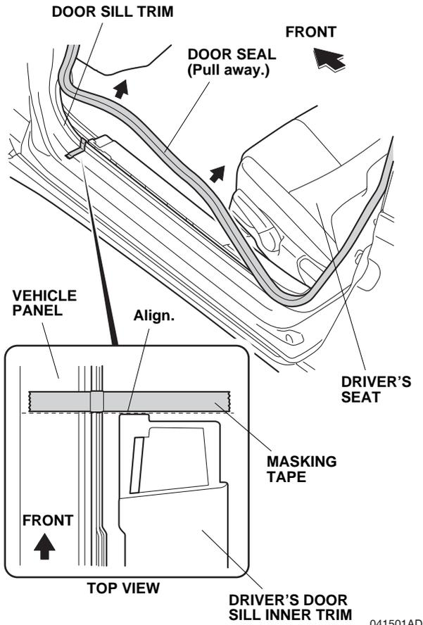
9. Apply a piece of masking tape to the vehicle panel. Align it with the front edge of the driver's door sill inner trim.
