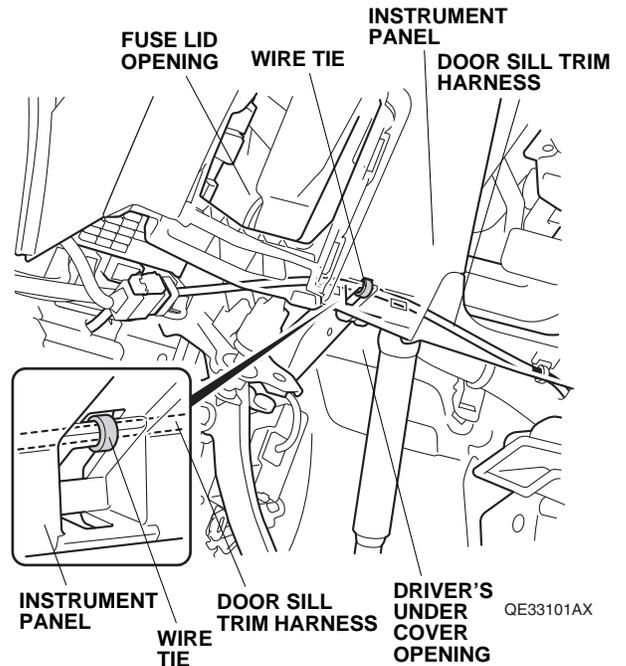
43. Route the door sill trim harness to the passenger side of the vehicle as shown.
