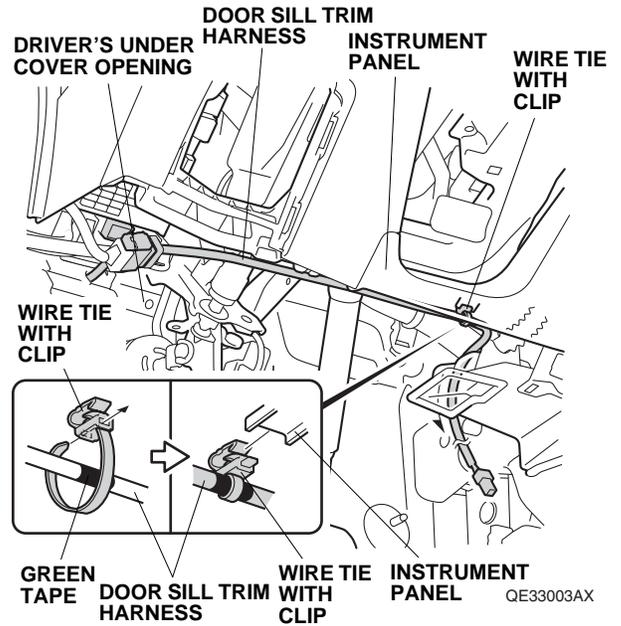
41. Attach one wire tie with clip to the green tape on the door sill trim harness, and secure it to the instrument panel.
