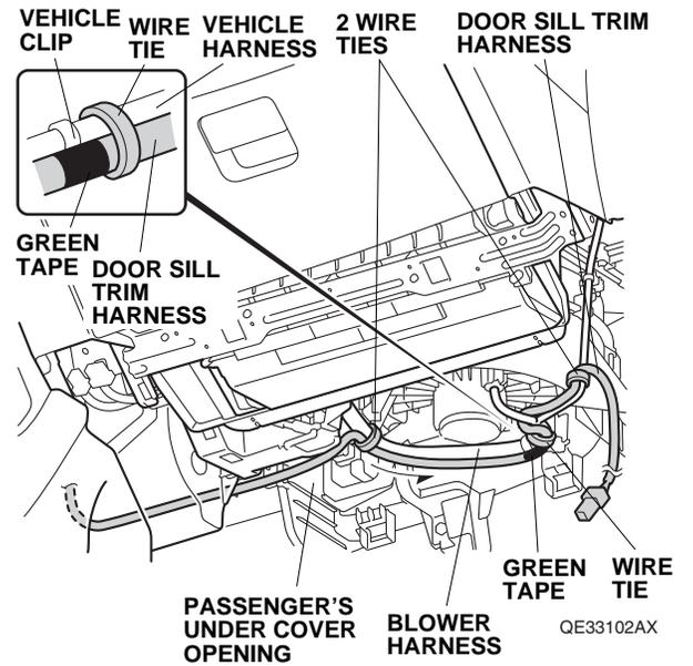
46. At the green tape, secure the door sill trim harness to the vehicle clip, and secure the door sill trim harness to the blower harness with one wire tie.
