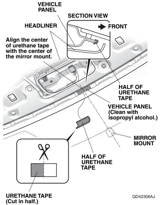
18. Using scissors, cut one urethane tape in half. Attach one half of urethane tape to the vehicle panel as shown. Be careful not to crease the headliner.
