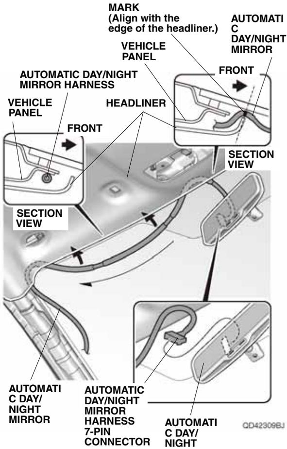
24. Gently pull back the headliner, and tuck the automatic day/night mirror harness behind the headliner. Align the mark on the automatic day/night mirror harness with the edge of the headliner. Be careful not to crease the headliner.
