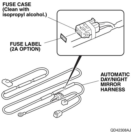
21. Attach the fuse label to the automatic day/night mirror harness fuse case.
