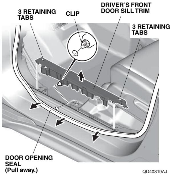
16. Pull away the door opening seal, and remove the driver's kick panel (two clips).
