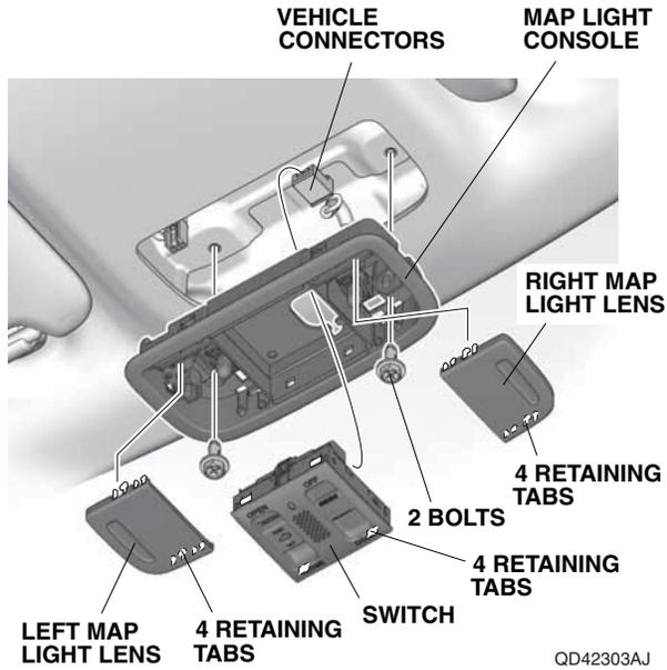
Without Moonroof: Remove the map light console (unplug the vehicle connector).
