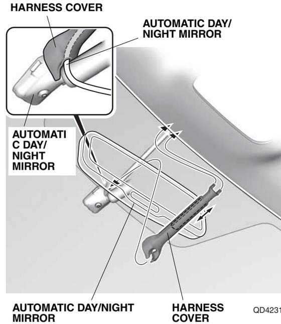
26. Route the automatic day/night mirror harness down the A-pillar as shown. Align the green tape on the automatic day/night mirror harness with the vehicle clip, and secure the automatic day/night mirror harness to the vehicle harness with two wire ties. Do not cover the installation holes of the driver's A-pillar trim.
