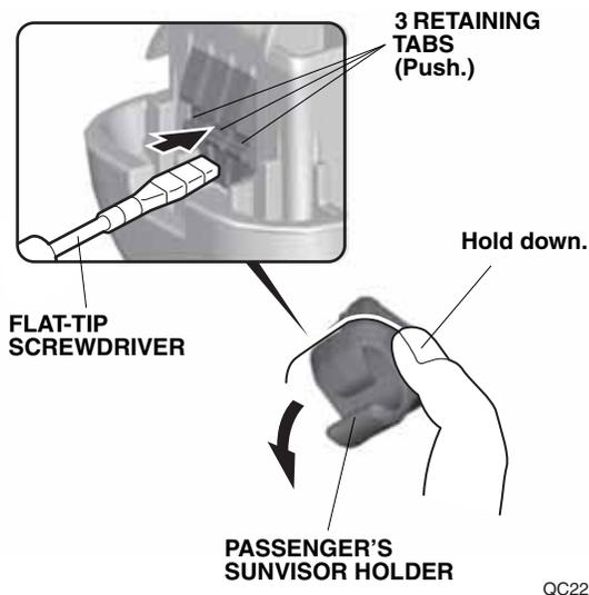
6. Remove the driver's sunvisor (unplug the vehicle connector):
