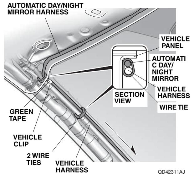
27. Align the green tape on the automatic day/night mirror harness with the vehicle clip, and secure the automatic day/night mirror harness to the vehicle harness with one wire tie.
