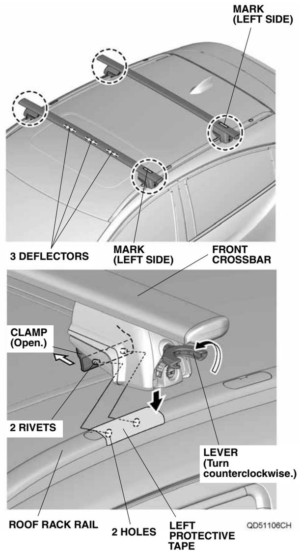
11. Align each rivet with the holes on the roof rack rail, and position the front crossbar. Make sure the crossbar is on the protective tapes.
