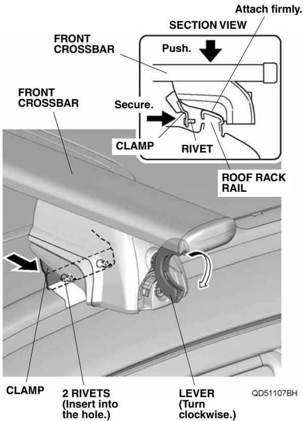
15. Lower the lever, and lock with key. Repeat on the other side.
