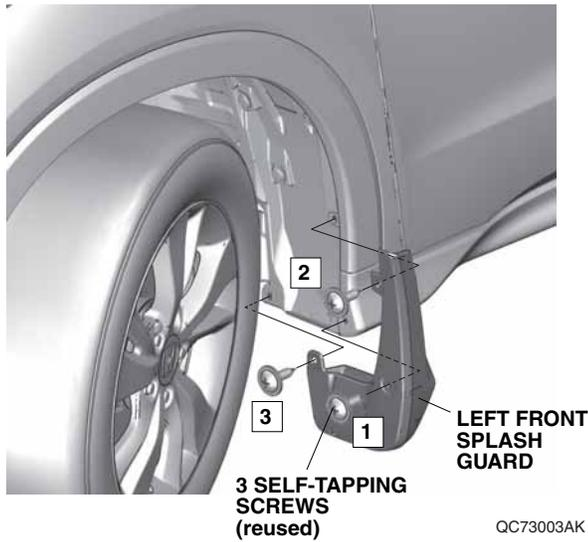
4. Remove the two self-tapping screws.
